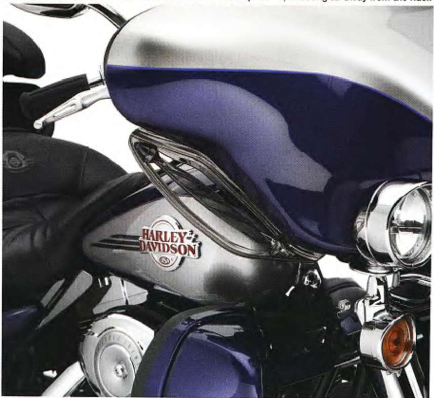
The deflector is now open to help direct more air toward the rider. Note the placement of the mid-frame air deflector near the frame's seat post.
