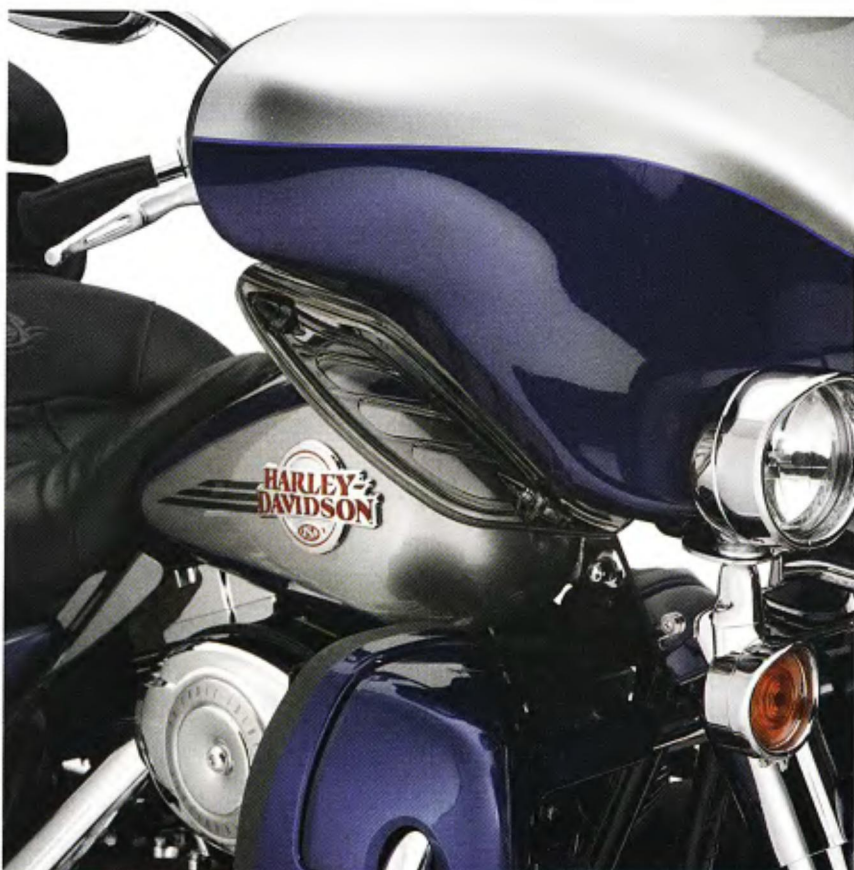
The adjustable air deflector is shown here in its closed position, directing air away from the rider.
