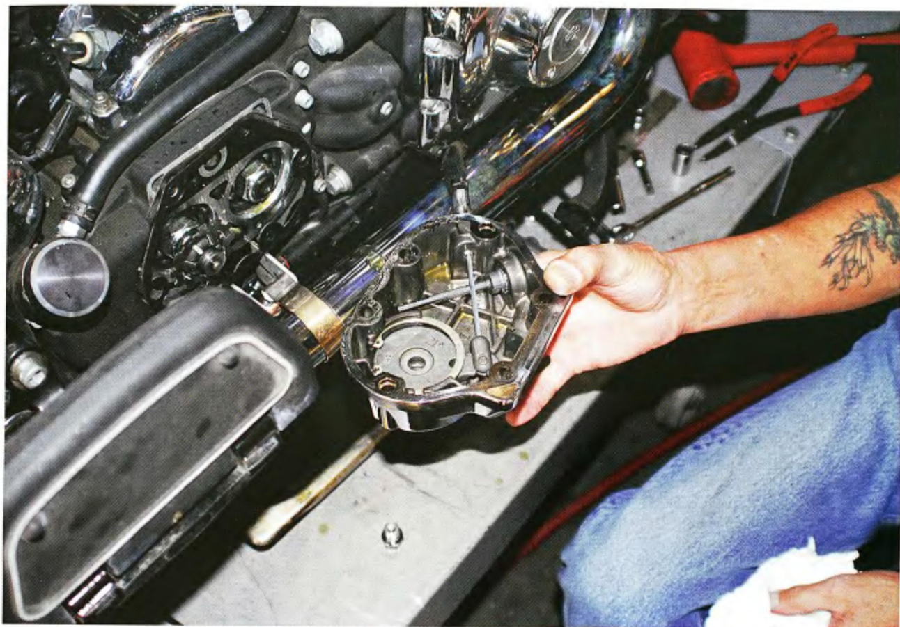
Clutch release cover removed revealing stock release mechanism.
