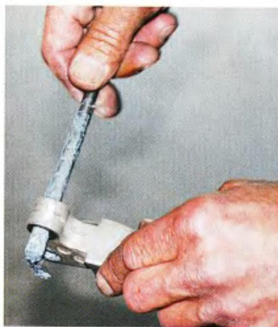
Apply grease to the clutch lever pivot and rubbing block and assemble lever.
