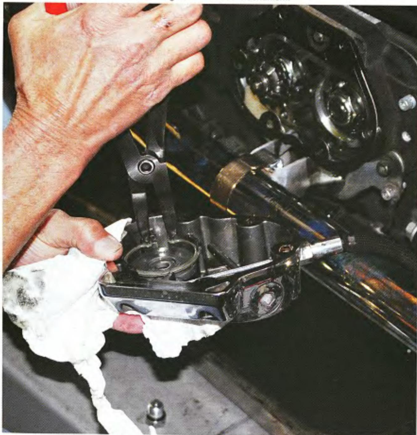
Remove the snap ring and the ball and ramp assembly.
