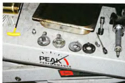
The Mueller Power Clutch compared to the OEM. Note that the ramps are located closer to the center, and the ramps are steeper than stock.
