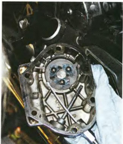
The outer ramp is installed and a dab of grease is used to lubricate and hold the bearings in place.
