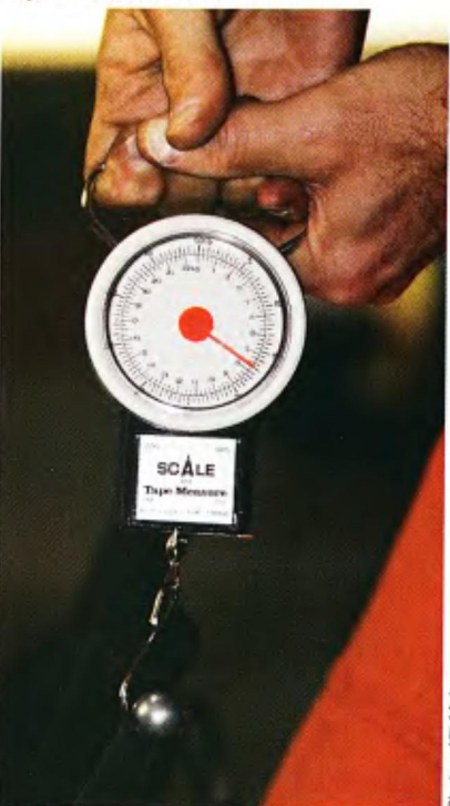
After the unit is assembled, there is a 5-pound decrease in pressure required to actuate the lever.
