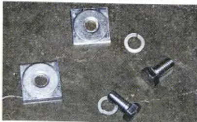
Two large nuts and two 1/2-inch bolts with washers secure the stand.
