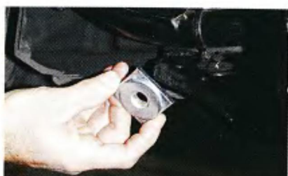
The nuts drop into the matching holes in the cross member.
