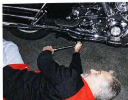
With the bike on the ground, torque the bolts to 35 foot-pounds.
