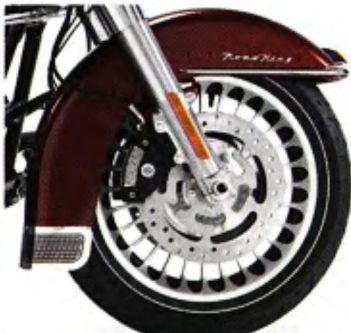
Larger, 17-inch wheels combined with model-specific Dunlop tires are used on the touring line except for the Road King Classic that retains 16-inch wheels and whitewall tires.
