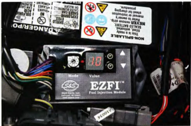
The EZFI, basic tuning knowledge, and a little experience makes EFI adjustments a breeze for most bolt-on modifications.
