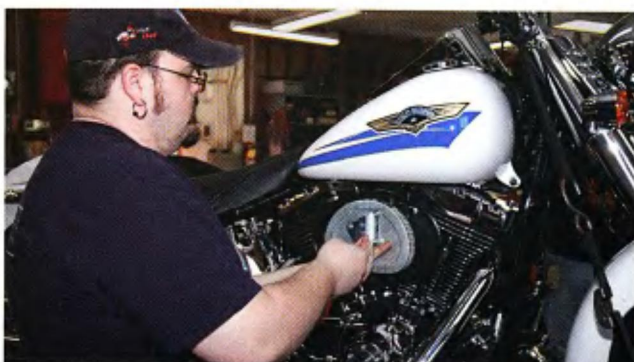
Technician-at-large Jamie "Cigar" Scott got the stock air filter off in less time than it takes to tell.
