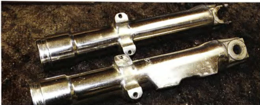
This is a set of late model Harley-Davidson sliders with a single-sided brake slider that someone had started trimming.
