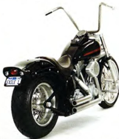
Creating a super clean look, the Exile bracket for bobbed fenders incorporates Lazer-Star turn signals and a LED taillight.
