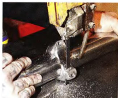
A band saw is used to whack off the big lumps of aluminum like the fender mounts.
