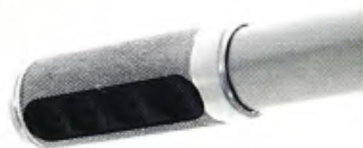
The billet "switchgrips" handle all of the lighting and starting chores from the handlebar.
