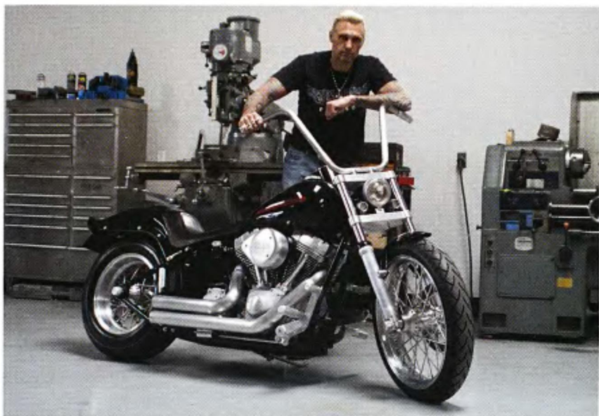
Russell with his latest endeavor featuring the brushed stainless SJP trees and headlight, and Exile apes with integral risers and internal throttle.
