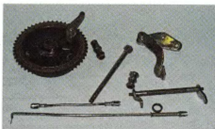
The mechanical drum brake parts removed.
