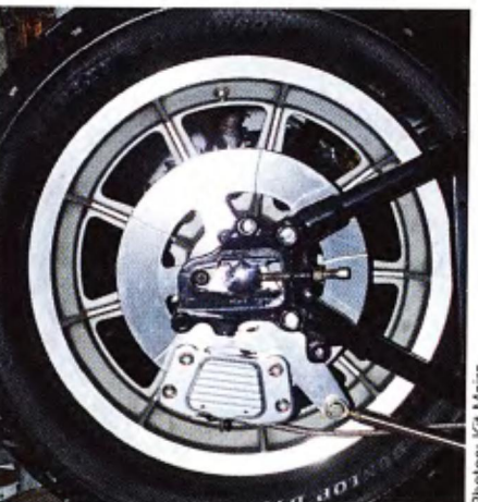
The installed brake unit.
