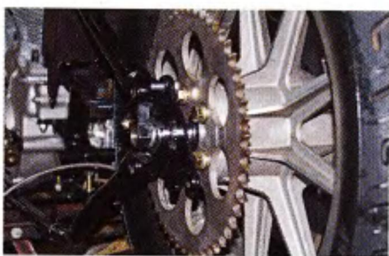
Left view shows the spacer, the adjuster collar and washer and nut.
