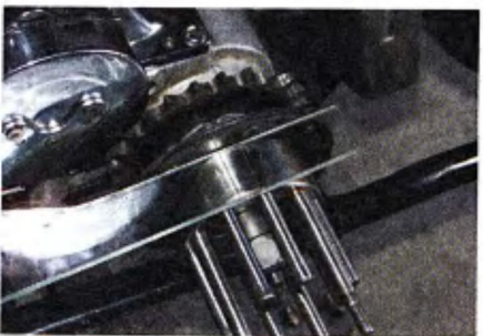
4 After alignment the oil bubble will be uniform across the bearing surface.
