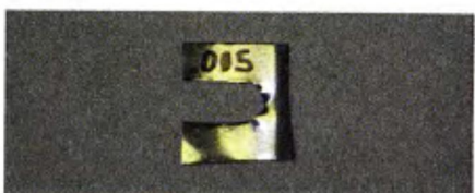
3 Cut some 1 1/4-inch squares of shim stock in various thicknesses with a cutout for the mounting studs to place between trans and plate.
