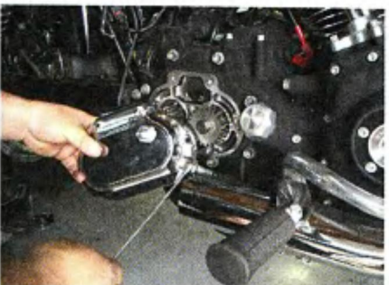
9 A new transmission cover is provided, so the existing clutch cable and mechanism must be transferred onto it.
