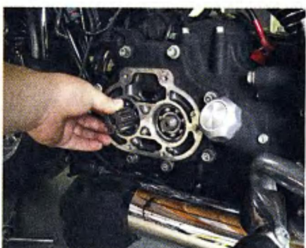
4 The provided main gear is placed on to the mainshaft and tightened using the special socket provided with the kit.
