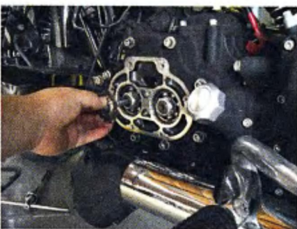
3 Installation starts with draining the transmission oil. Open the transmission cover next and remove the oil slinger and the nuts from the mainshaft and countershaft.
