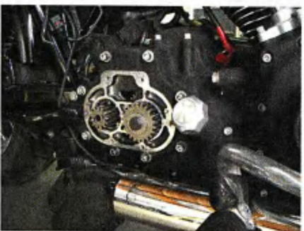
8 The counter shaft bolt is installed and tightened to specs.
