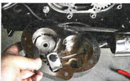
10 Shown in the center of the cover is the sliding reverse gear that will be used to engage reverse using the lever outside the cover.
