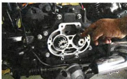
6 The counter boss nut is then installed on the counter shaft and torqued before allowing the counter gear to be installed.
