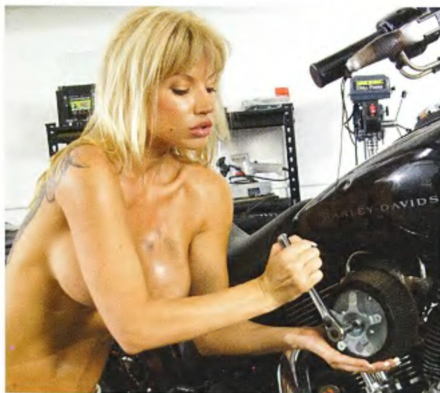
6 Under that top cover, the one on the bike, was a mounting bracket, which also had to come off. Angie used a ratchet and Allen socket to get it off.
