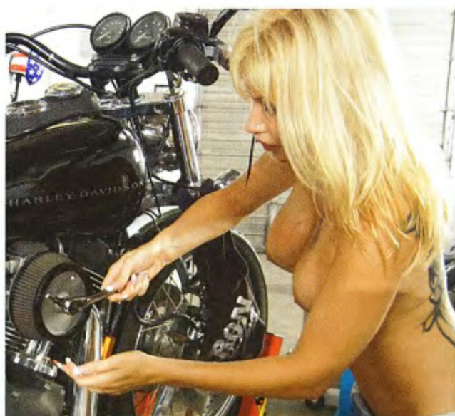
7 Angie finally got down to the filtering element's mounting screws. Three screws later and the filter was off.
