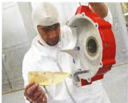
9 The masking is removed and the powdercoating is completely inspected.
