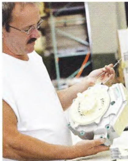
4 Any area where powdercoating is not wanted is masked. They use silicone plugs in all of the bolt holes. Because powdercoating is several times thicker than paint, surfaces that are bolted together need careful attention to keep them free of any powdercoating.
