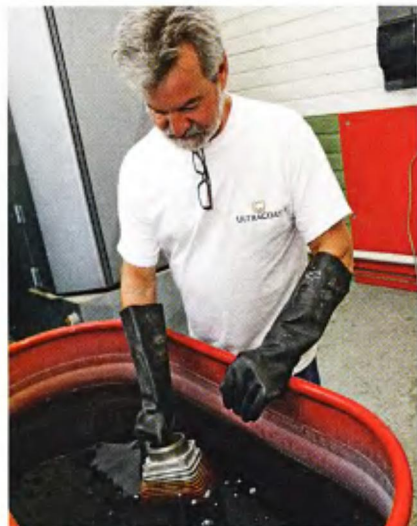
2 Just like a good paintjob, the quality of the powdercoating is only as good as the prep work. First, UltraCoat starts with a chemical cleaning.
