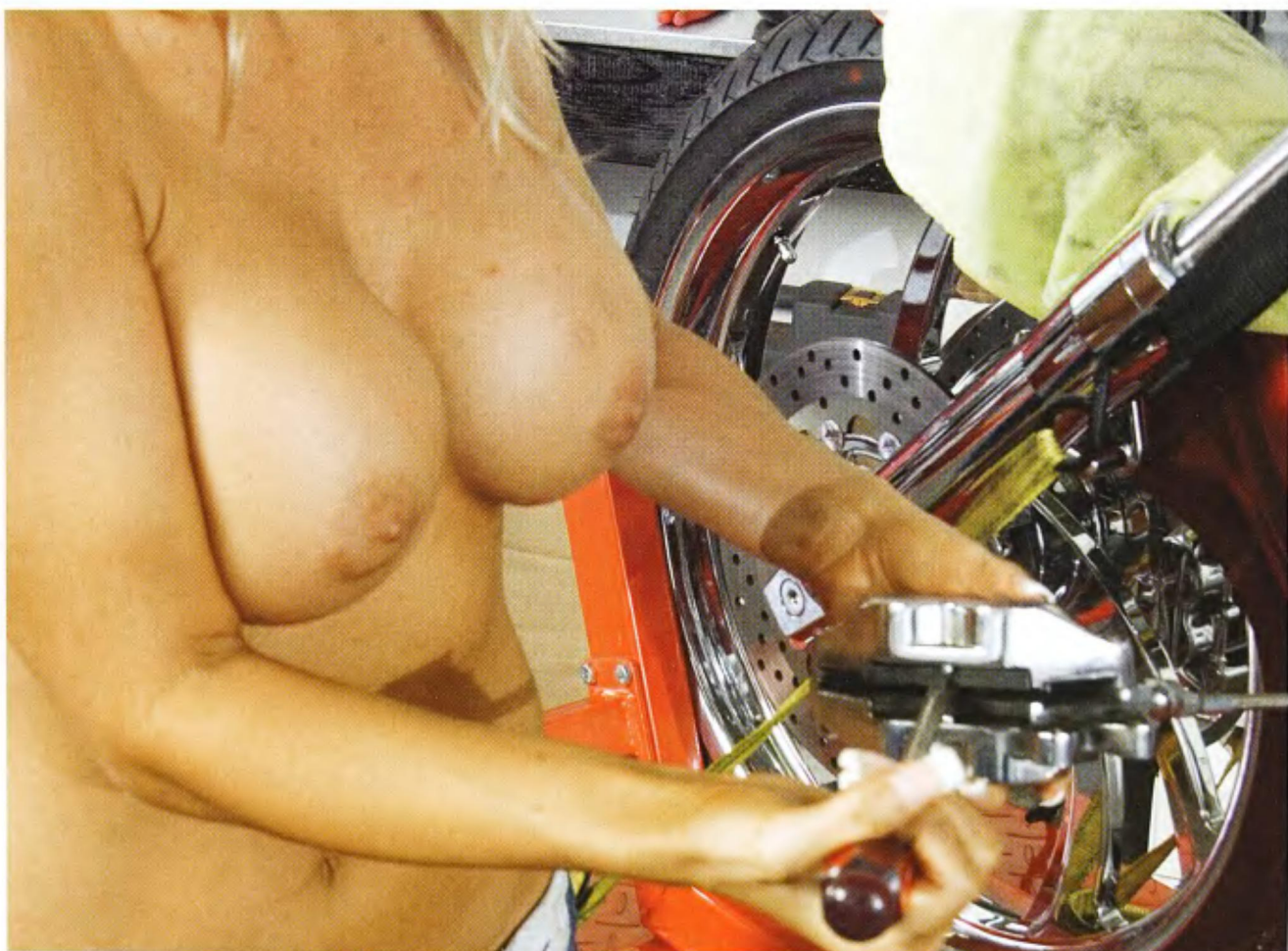
8 Using a good-sized screwdriver, Angie spread the pads apart, forcing the caliper's pistons into the caliper body so she could fit the caliper down over the rotor. With that, the Torx mounting bolts were each given a drop of #242 Blue Loctite and installed. After that, she squeezed the brake control a couple of times to seat the pads.
