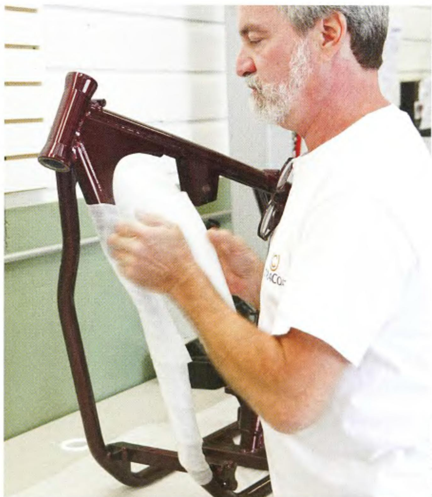
10 After the powdercoating is finished, the part is wrapped with a soft fiber cloth, boxed and shipped back to the customer. All of this takes about 10 days. The cost is competitive with painting, but the finish is far more durable.
