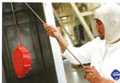
8 After the part is cured, it has a nice shiny finish. It then needs to cool for one hour or so.
