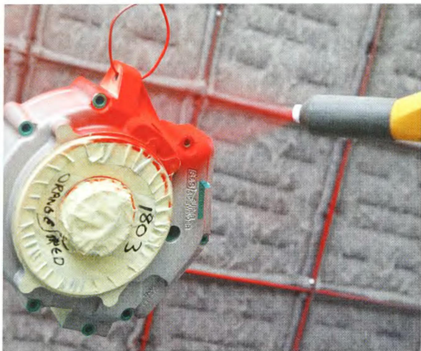
6 When the raw powder is first sprayed on the metal, it has a course dull appearance. The special electrostatic spray gun assures good coverage.
