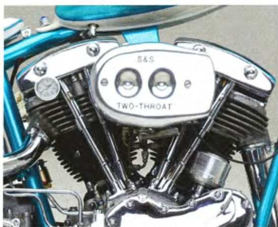
Rare S&S dual-throat carburetor/air cleaner.
