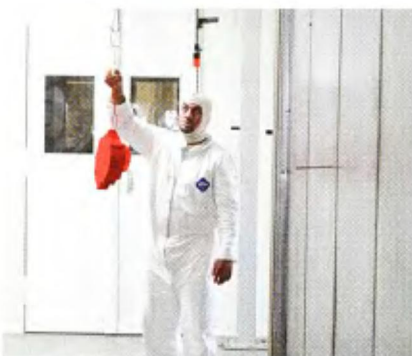
7 From the spray booth, the parts are pushed into the curing booth. They'll be heated to 390 degrees for about 10 minutes.
