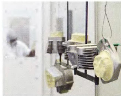
5 The parts are then hung from an overhead track that runs from the prep area to the spray booth and on into the curing oven. Over the years, they have made a lot of special fixtures to hold motorcycle parts during the spraying and curing operation.
