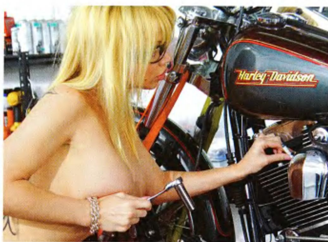
8 Being careful is one of Angie's hallmarks, so to prevent cross threading, she screwed the new spark plug in by hand until it was finger tight. Then she finished tightening it with her ratchet.
