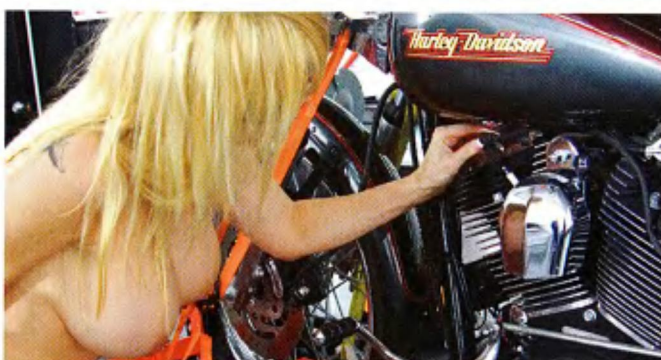
9 Being careful not to stretch the connector on the end of the spark plug wire, she firmly seated it on the tip of the spark plug.
