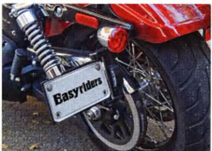
Harley chose to side-mount the license plate on a hinge.
