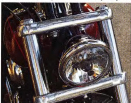
The 46mm fork tubes with billet trees look great and provide excellent tracking.
