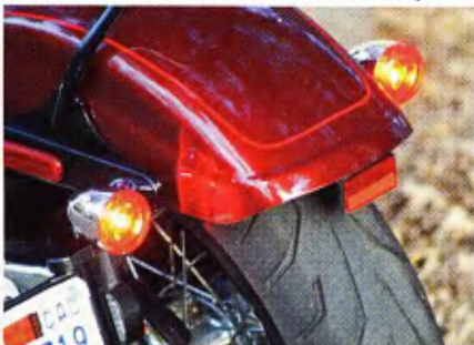
Harley integrated the stoplight into the tail-light to clean up the rear section.
