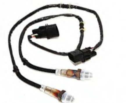
3 The new oxygen sensors were installed in place of the stock units in the exhaust head pipes.
