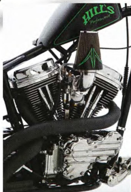
The Evo-pan motor started with a bottom end taken in trade from one customer and cylinders and heads from other trade-outs.
