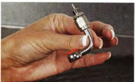
7 The fitting has a small tube sticking out. "It fits into the end of the hose, which makes the seal," says Angie.
