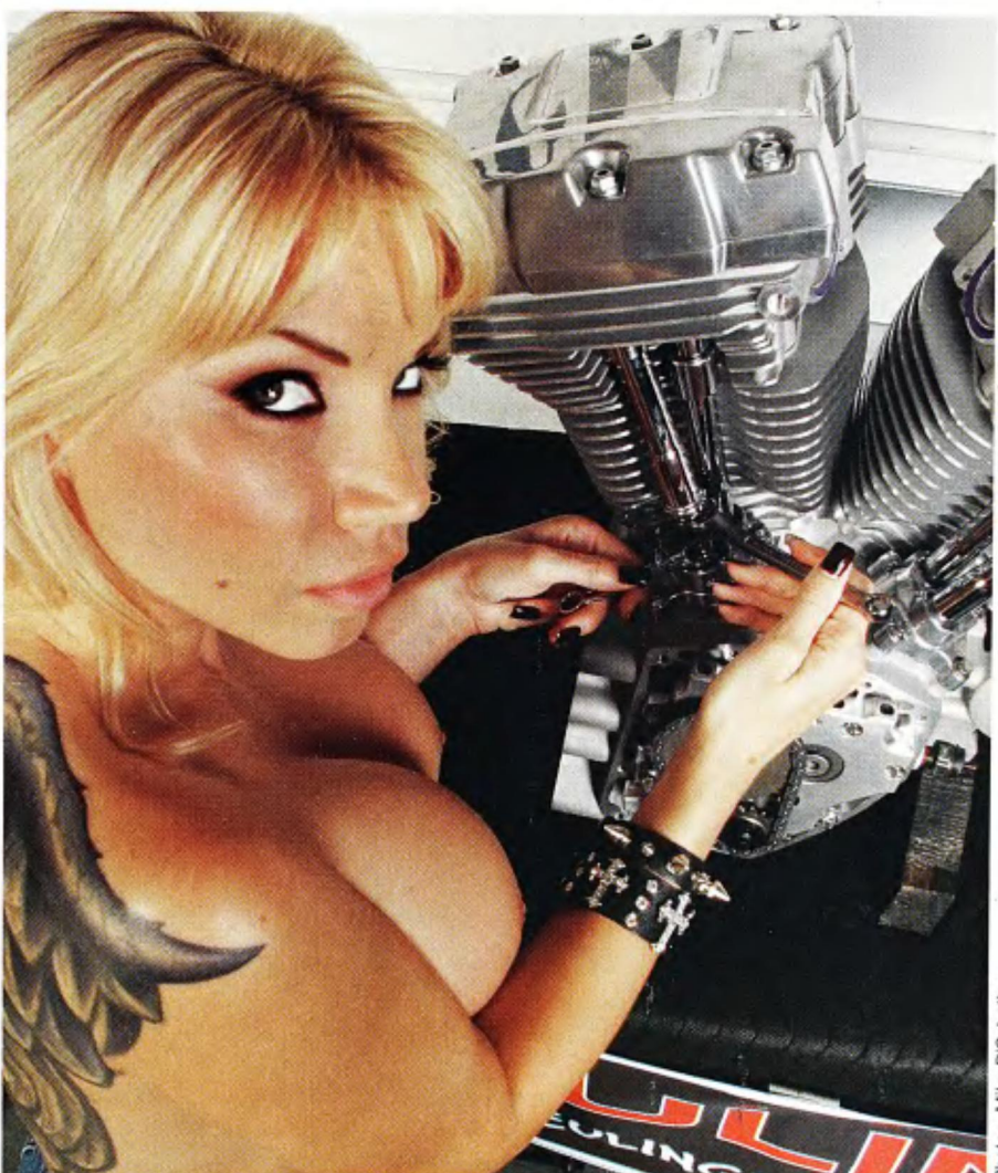
8 For the reassembly Angie says, "You need to be very careful when you adjust the pushrods; make sure the lifter is on the heel of the cam and adjust the pushrod to 3 1/2 turns after all of the slack is taken out. Then let the motor settle for 20 minutes before you rotate the crankshaft. This lets the lifter leak down so that the valve won't hit the top of the piston."
