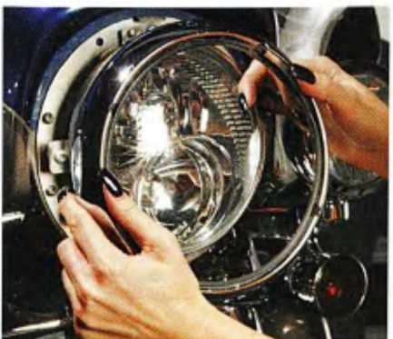
4 Once she got it off, the headlight ring mounting screws were exposed.
