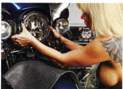
3 Angie says, "The trim ring is a tight fit, so gentle but steady force is needed."
