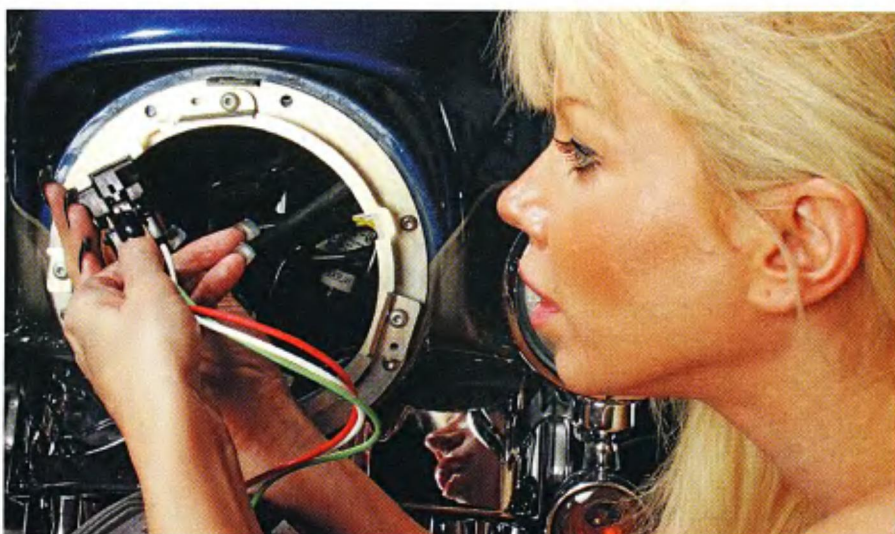
8 For the reassembly Angie says, "You need to be very careful. Push the headlight's plug all the way in; it is a tight fit."
