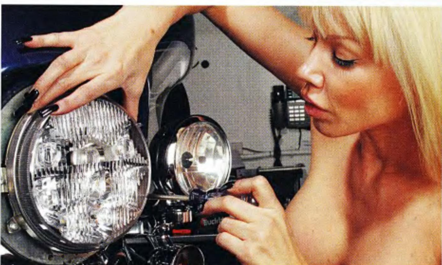
9 In putting the whole thing back together Angie says, "Make sure that you line up the tabs on the headlight before you screw the mounting ring down tight."
