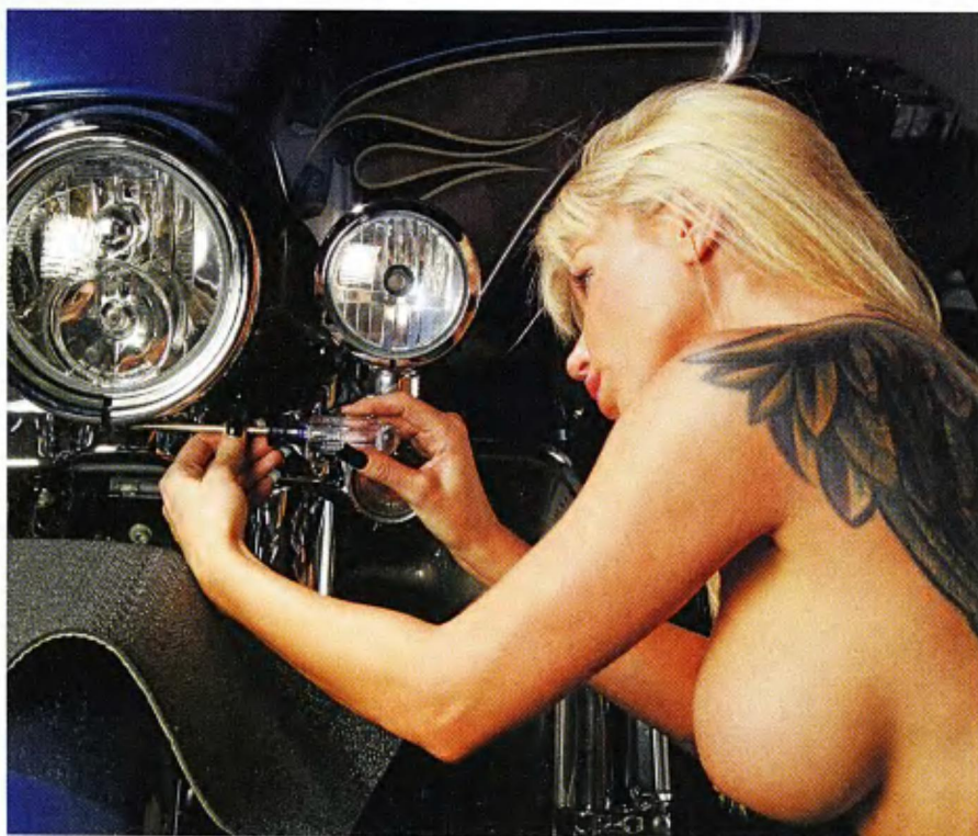
2 Angie used a phillips screwdriver to remove the headlight trim ring. She says, "If your bike has a custom headlight, you might have a bunch of screws to un-do."
