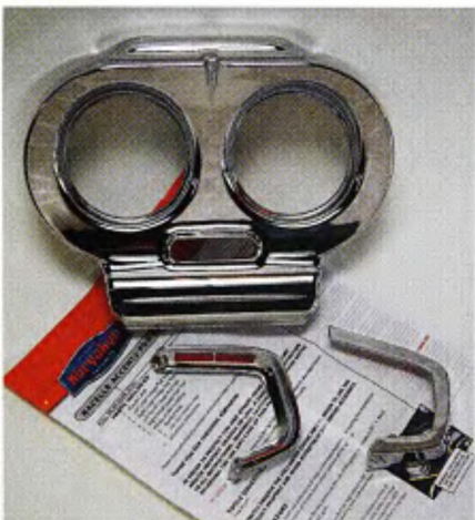
8 The Küryakyn chrome dash trim kit. It includes the gauge housing cover and four accent pieces that fit around the center switch housings.
