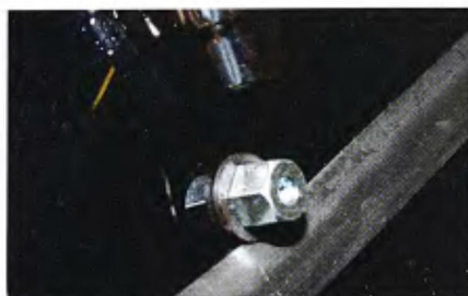
5 To install the chrome windscreen trim, four of the attaching screws are removed and replaced by these stand-offs.
