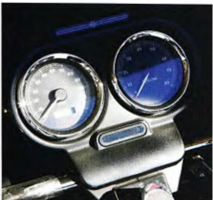
9 The Road Glide has a rather bland-looking dash console. The chrome trim pieces fit over the factory parts nothing is disassembled.
