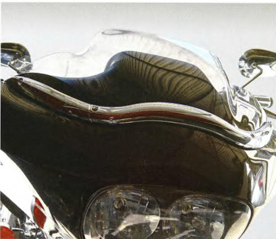
7 The completed Sport Windscreen and chrome trim installation, it gives the Road Glide a very slick look.
