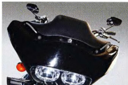
3 The Kuryakyn Sport Windscreen and chrome windshield trim. The chrome trim will also fit on the factory windshield.
