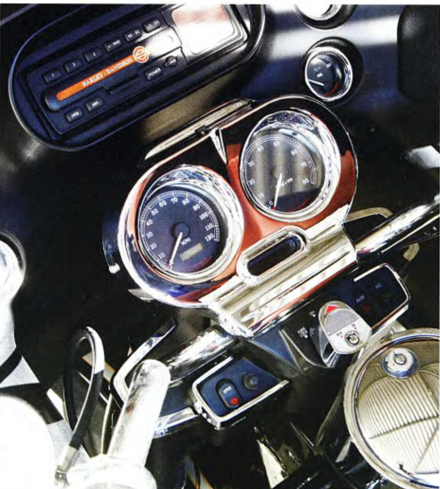
10 The bright work installed, check out our new dash and switch housings. The gauge cover is held in place with two stainless steel screws that thread into the factory holes in the stock dash. The trim pieces on the switch housings are secured with high-strength double-sided sticky tape.
