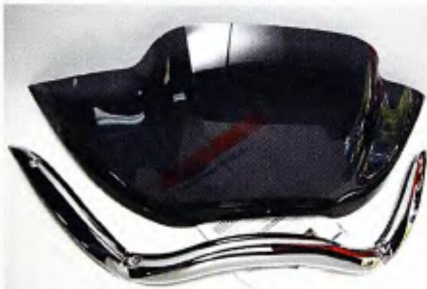
2 The Kuryakyn Sport Windscreen and chrome windshield trim. The chrome trim will also fit on the factory windshield.
