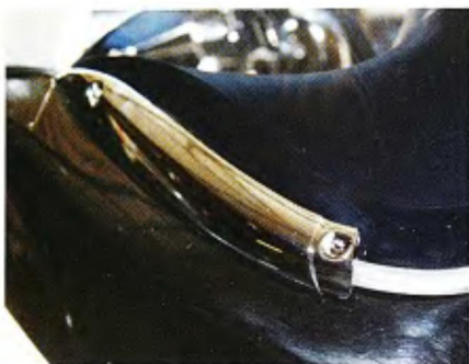
6 The chrome trim is made in three sections. The two outer pieces are installed first, then the center section. They are secured to the stand-offs with small Allen head screws.
