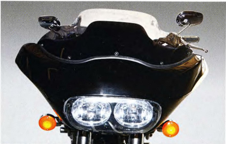
4 The factory windshield comes off easily; just remove five screws. The screws and weather stripping are reused with the Kuryakyn Sport Windscreen.
