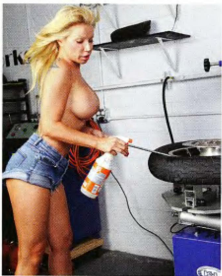
5 "Use a good tire lube to prevent chafing the tire's bead when you insert the tire iron," Angie cautions.
