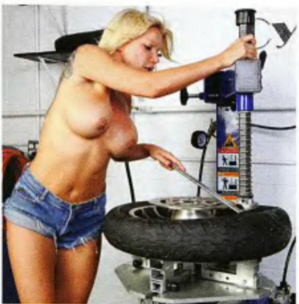
6 The shoe on the end of the machine's arm lifts the bead over the rim as the turret rotates the wheel. Can you spot the turret in this photo?
