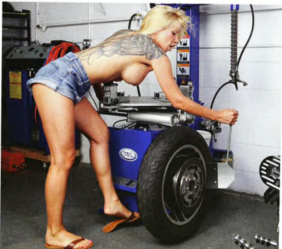
3 Angie used the bead breaker attachment to get into the tire. She said, "This is so much easier than a tire hammer and bar. I can save my energy for fun stuff."
