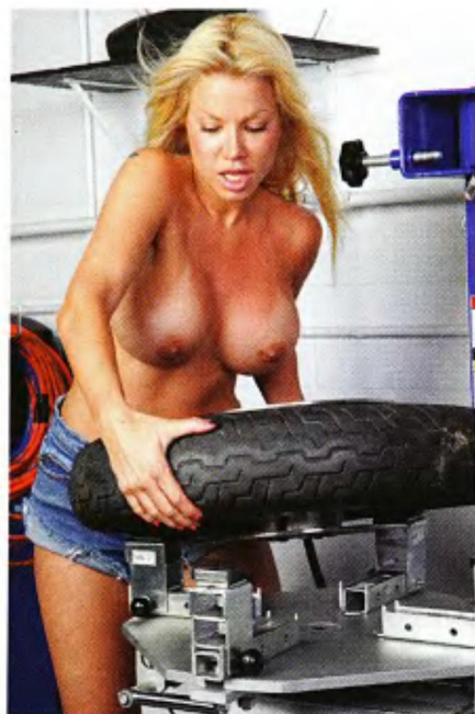
4 Next she had to mount the rim on the top of the machine's turret. "Make sure that you get the machine's lugs inside rim's edge, then tighten them down," she says.
