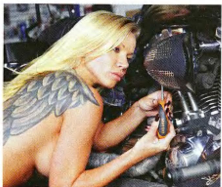
8 Angie rotated the filter's inlet forward and tightened the screw clamp. "The cool thing about this filter is you can point its inlet in any direction," she explained.
