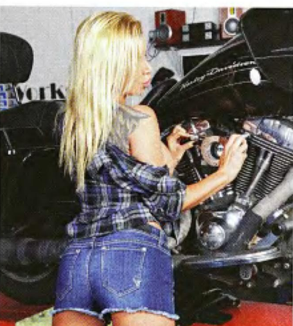
4 She put all of the mounting screws in finger tight. "Make sure that all of your hardware started in the threads before you tighten them," Angie cautions.
