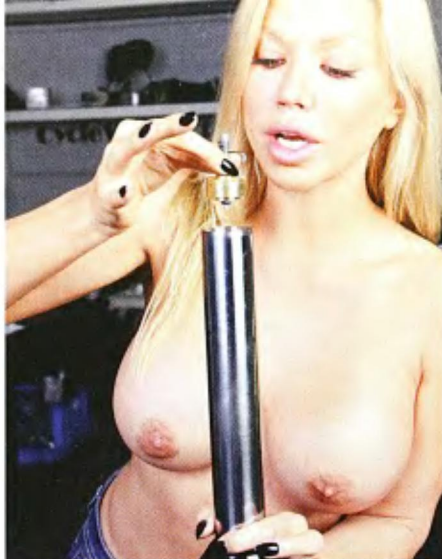
12 She carefully dropped the Race Tech emulator valve into the top of the tube. This is the part that makes a regular fork into a great fork, so be careful," Angie cautions.
