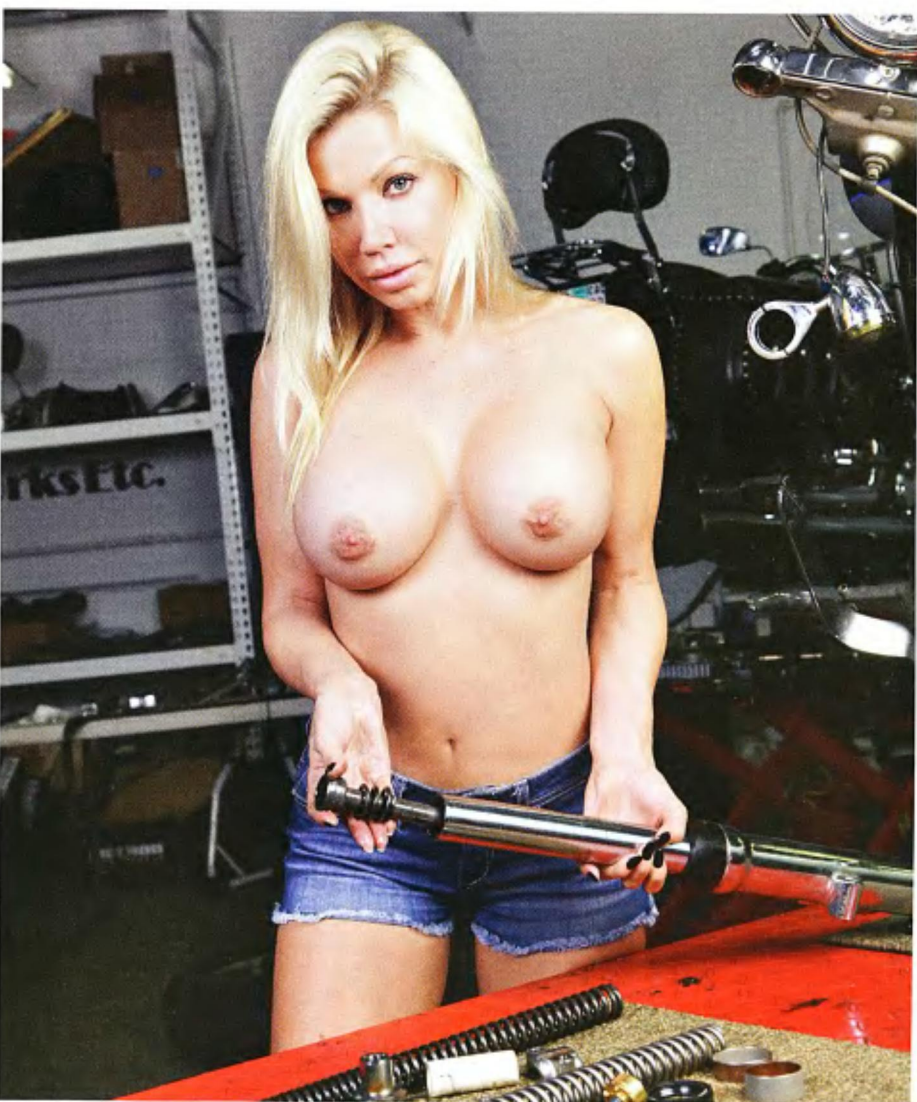
8 Angie then turned the tube upside down and removed the damper rod assembly.
