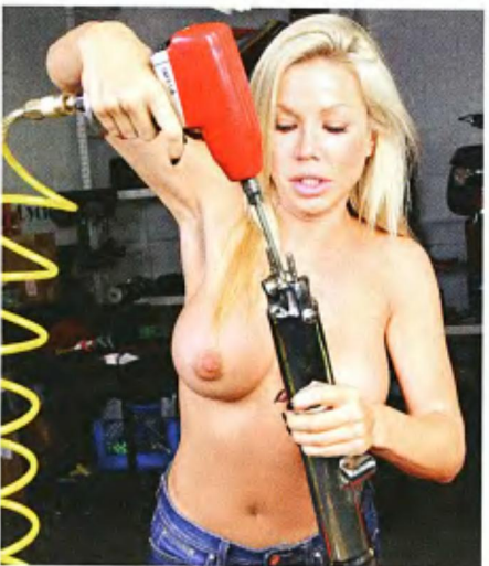
7 Angie used an air wrench to remove the damper rod bolt. "I really like air tools, they make the job go fast," she said.
