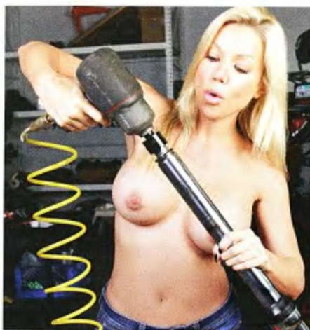
4 "The Wide Glide tubes top caps take a big wrench and a bit of air to muscle them off," says Angie.
