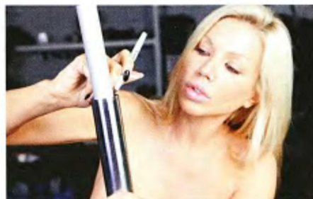
14 The Race Tech kit uses an aluminum tube to set the fork's ride height; Angie marked its edge for cutting.
