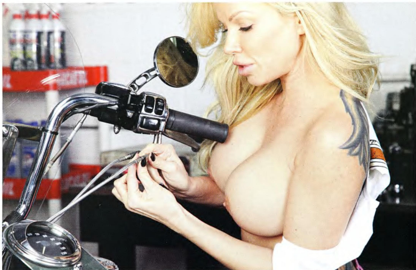
5 On the right grip, you need to loosen the throttle and idle cables. They have adjusting screws about 6 inches down from the grip.
