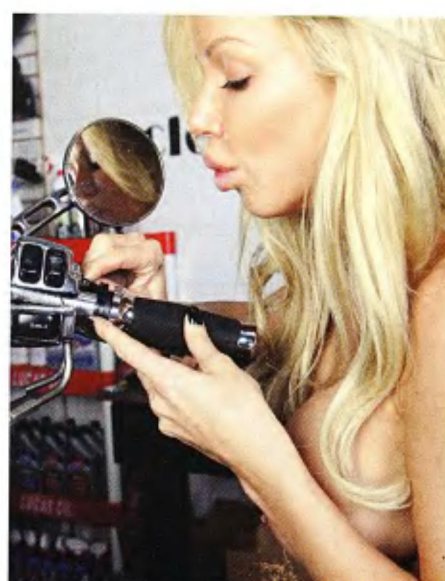
10 As she was fitting the cables onto the throttle grip, Angie said, "Make sure you don't bind them with the edge of the switch housings."
