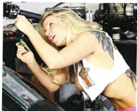
4 "There are two screws in each switch housing, one on the top and one up underneath," explains Angie.
