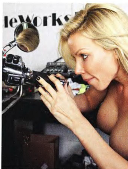
9 In putting the whole thing back together, Angie says, "Make sure that you line up the end of the grip and the cables before you push it in."
