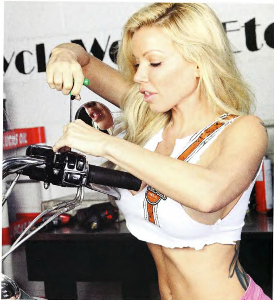
1 Angie used a hex driver to remove the upper screws from switch housings from the handlebars. "Because of their internal wiring, you aren't going to completely remove the housings, just lift them off the end of the grips," she says.
