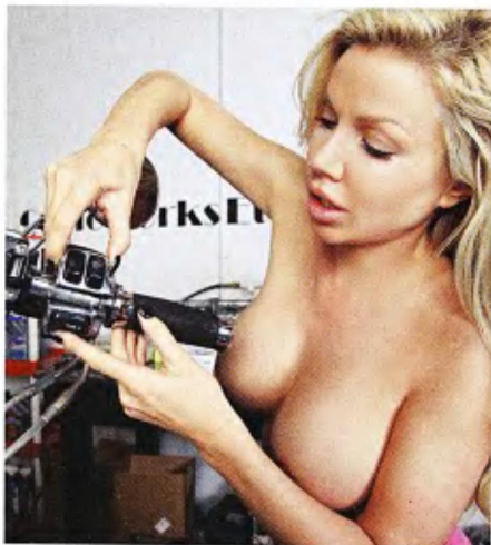
11 Angie fit the two sides of switch housing over the end of the grip.
