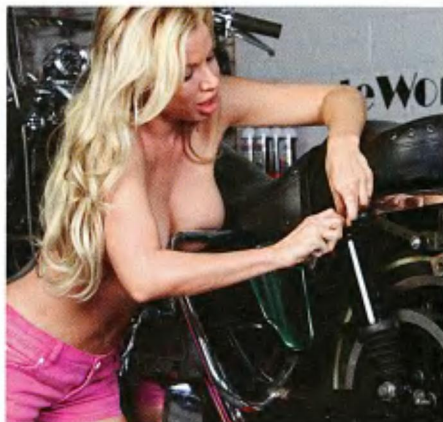
10 Angie installed the bottom bolts first, and then lowered the bike jack till the top bolts lined up with the holes in the frame.
