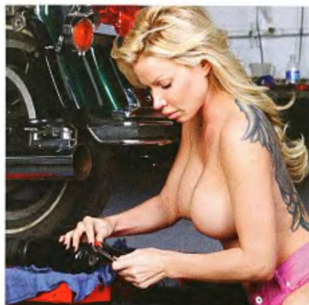
7 The air line fitting must be transferred to the new shock. "The fitting is made out of brass, so don't over tighten it," Angie cautions.
