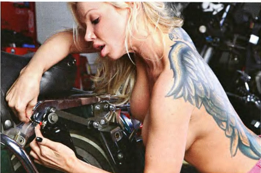
11 Angie inserted the air line into the fitting on the shock and one side was finished. Then it was just a matter of installing the other shock and pumping 5 pounds of air into the system.
