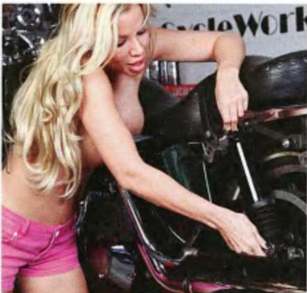
9 Putting the new shocks on, Angie says, "Make sure that you start the bolts with your fingers, you don't want to cross-thread these bolts."
