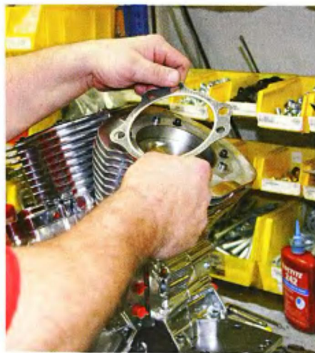
2 Installing the head gaskets.
