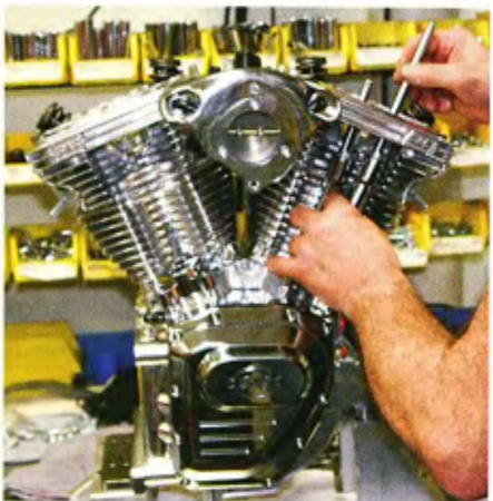
7 Dropping in the push rods.
