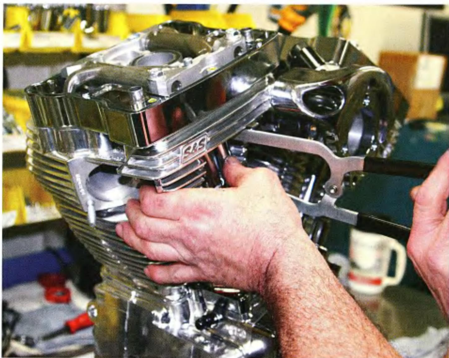
8 Installing the push rod keepers.
