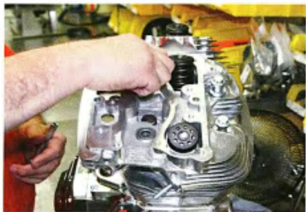
5 Installing the head bolts.
