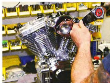
12 Torquing down the back plate bolts.
