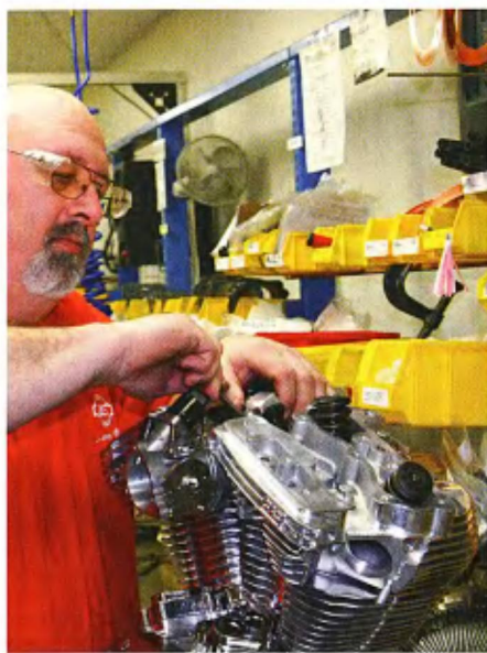
10 Tightening the manifold flange.
