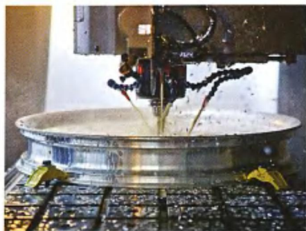
3 Water jets keep that drill bit cool. Don't try this at home!
