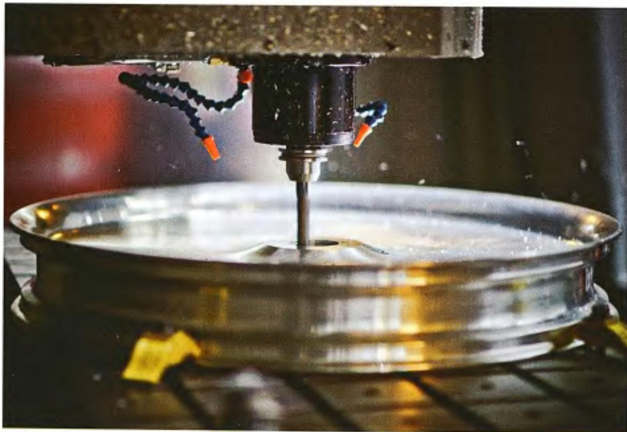
1 Your Renegade wheels started off as big chunks of billet aluminum.
