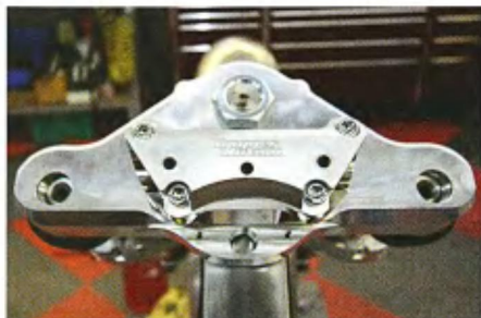
4 With a 3-inch forward stretch we'll make some special bars with extra pull back. Our Bagger Nation Super Riser Clamp will hold on to any design we can dream up.
