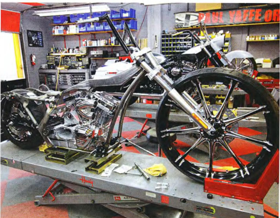
9 The backbone stretch on the frame will be hidden by a custom gas tank. Our goal is to make the bike with flowing clean lines that just look longer and somewhat larger than stock. Other than the sweet, arched front downtubes, you can barely see the difference between the new frame's geometry and the just raked for a 23-inch wheel 2012 H-D that sits on the lift behind it.
