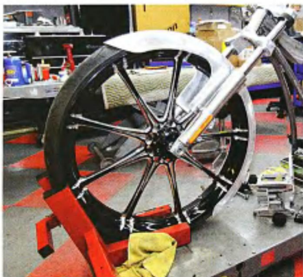
5 B Cool Products made the 30-inch front fender out of aluminum to save weight due to the size of the spinning. Randy also doubled the wall thickness to reduce flex.
