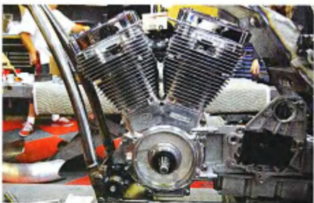
6 The S&S 111T hybrid engine looks sweet show polished. We opted for closed port EFI as well. Now it's starting to take shape once we put it on its feet! With a pedigree like S&S you know this bike will not only show, it will go as well. We conservatively estimate 120 HP outta this bad boy!
