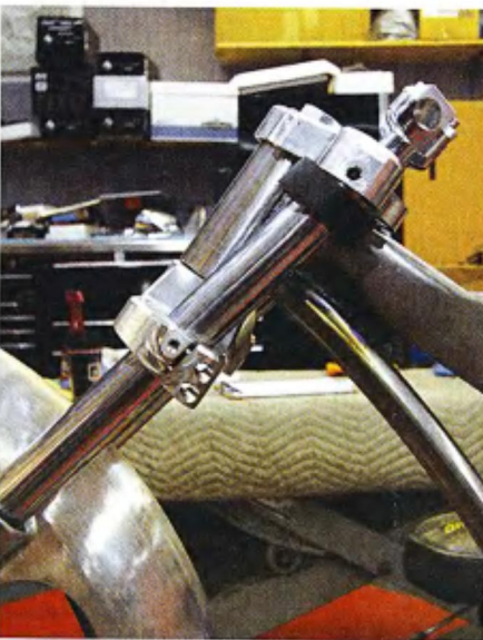
2 We added 12 degrees of rake in the neck to correct the trail so that the bike will handle beautifully even with the monster 30-inch hoop.
