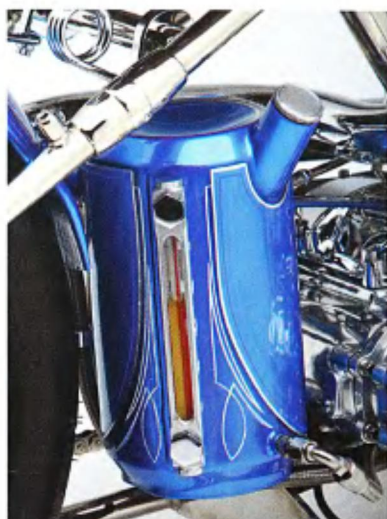
Jutt found a sight glass from an industrial boiler and put it in service on the side of the tank.
