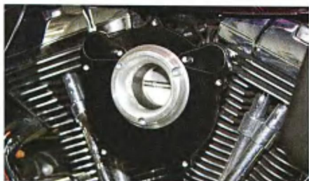
8 The two breather cover plates are installed over the breather bolts in the back plate recesses.
