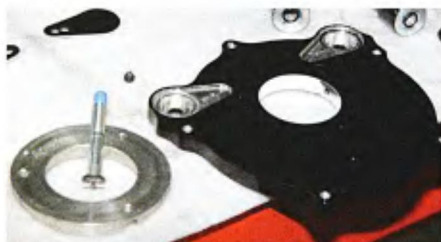
6 The RC Components back plate has breather passages that connect through the included hollow mounting bolts to the breather ports in each cylinder head. We put a couple of dots of medium thread locker on each bolt before threading them.
