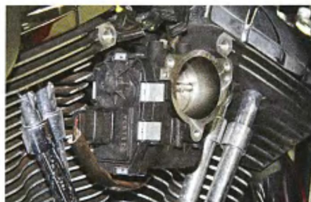
5 This is our starting point; all of the factory parts have been removed. The new gasket from the RC air filter kit will be fitted to the throttle body's air horn.
