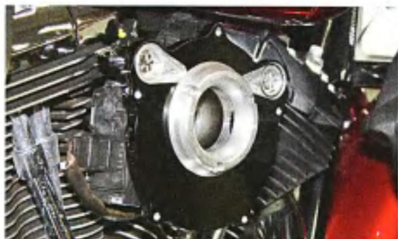
7 The two breather bolts are loosely installed with their spacers to fit the back plate to cylinder heads. Three Allen bolts are used to secure the air guide and back plate to the throttle body. We put a drop of medium thread locker on each of them and tightened them to 10 inch-pounds; we then tightened the two breather bolts to 50 inch-pounds.
