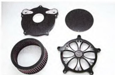
1 The Majestic air cleaner kit is complete down to the last detail. All needed parts, gaskets, hardware, and instructions are included.
