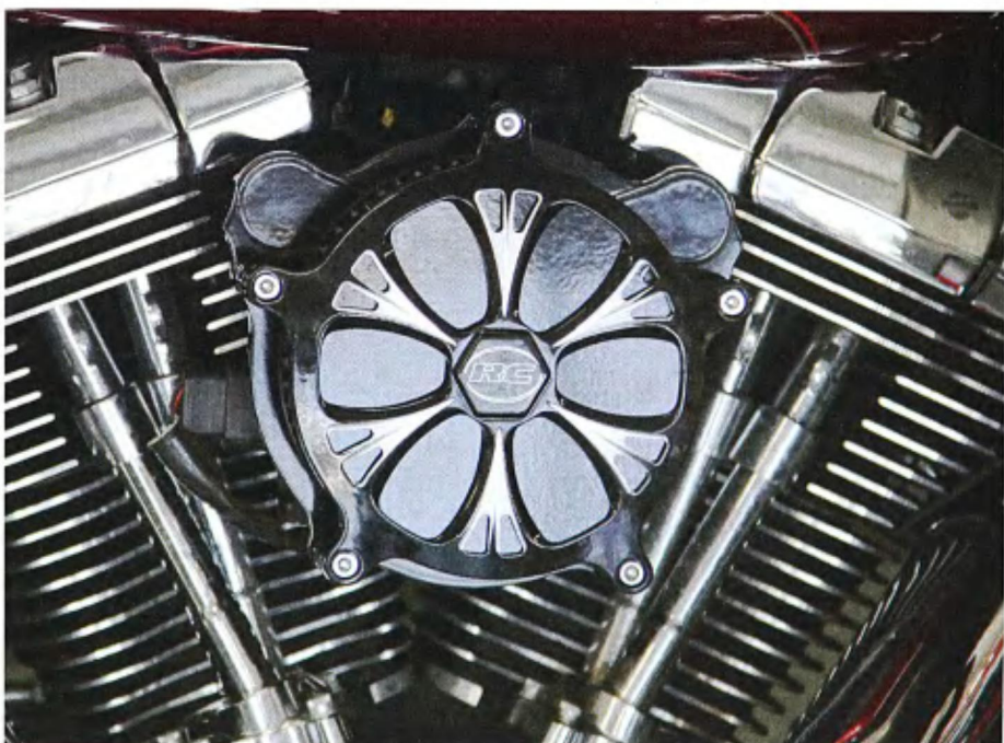
10 The finished installation, the air cleaner's gloss black powdercoating and raw aluminum finish matches the motor's cylinder fins.
