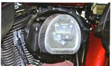
4 This is the factory filtering element on our 103-inch motor; it is the same as what was used when the motors were only 96 inches. It is good at cleaning the air it just lacks a bit in volume.
