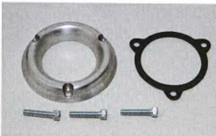
2 The air intake guide ensures that the transition between the filtering element and throttle bore is smooth and turbulence free.
