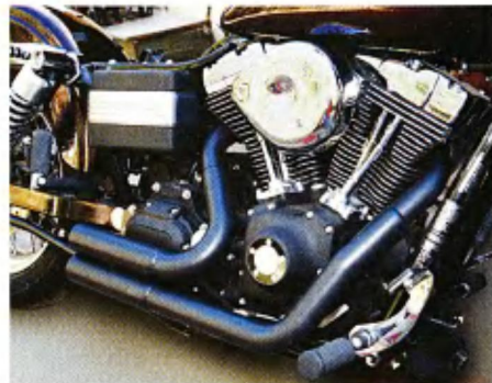
10 The Vance & Hines head pipes fit nice and close to the motor. We routed the oxygen sensor wires back to their connectors, making sure they were out of harm's way.
