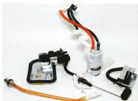
16 These are the parts that live inside of a 2007-up Harley gas tank: fuel pump, fuel filter, fuel gauge-sending unit and output line. The output line actually threads in from the bottom of the tank.
