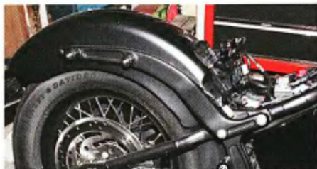
8 The fender assembly is secured with four bolts, two on each side. The plastic tray that holds the fuel injection computer must also be disconnected from the fender's front lip.
