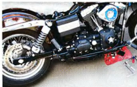
7 Once the electrical connectors were disconnected, removing the pipes was just like any other Harley. The stock muffler bracket was unbolted from the rear of the transmission.
