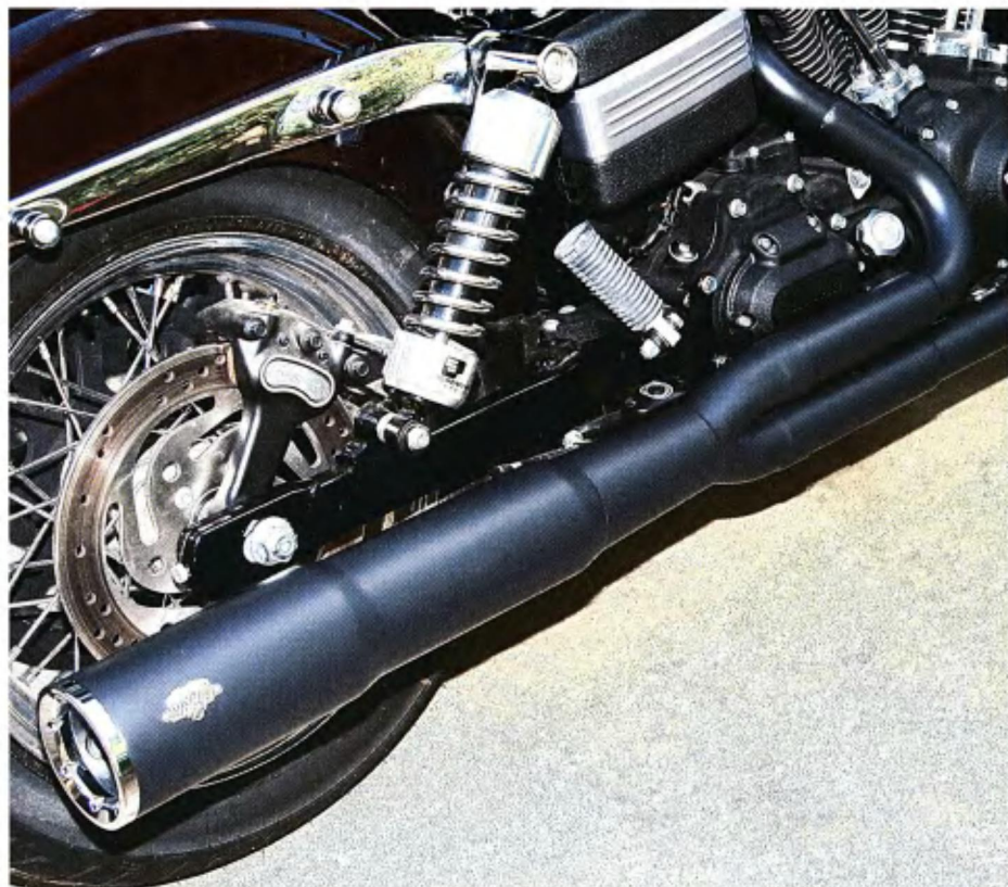
11 The muffler slips over the ends of the head pipes and is bolted to the new mount. With this, the install was finished.
