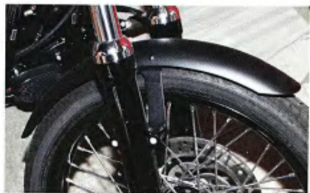
4 On Softail models, the front fender is attached with four Allen head bolts.
