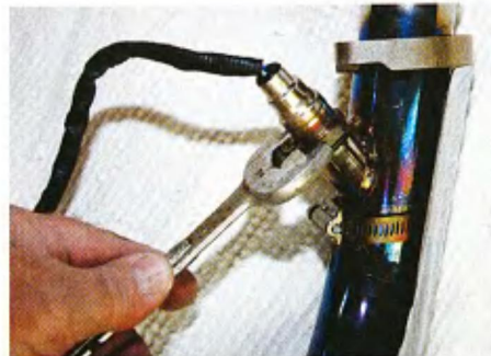
9 The oxygen sensors must be switched from the stock head pipes to the new pipes. Before screwing them in, we swabbed a little anti-seize on their threads. Handle them carefully, they are expensive.
