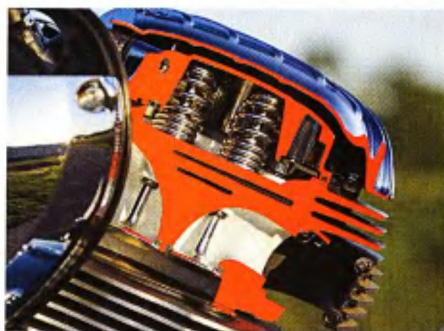
The overhead valves and ports offer high-flow rates, which translate into more usable torque at the output side of the crankshaft.
