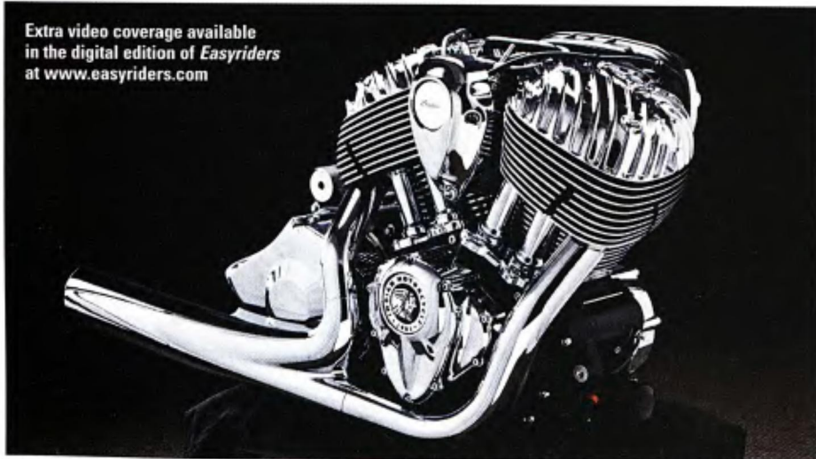
The Thunder Stroke 111 motor closely resembles the iconic Indian Chief V-twins from the 1940s. It is fitted with multi-directional finned rocker boxes, parallel pushrod tubes, downward pointing exhaust pipes and a left-side air intake.
