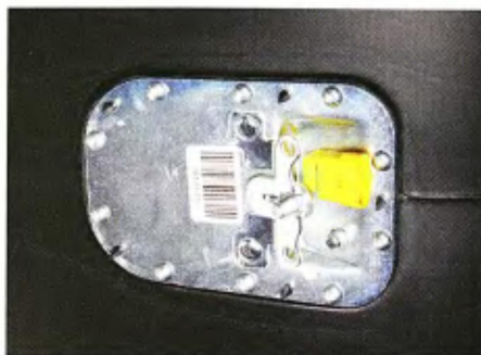
14 The fuel tank's center cover is attached with ten small screws. Harley recommends using new ones whenever they are removed.
