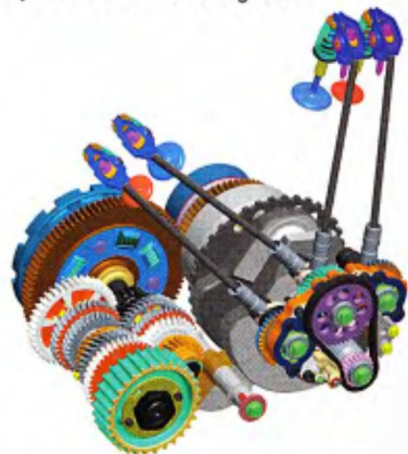
The camshafts' drive system uses a unique hybrid chain and gear set to rotate the motor's camshafts.
