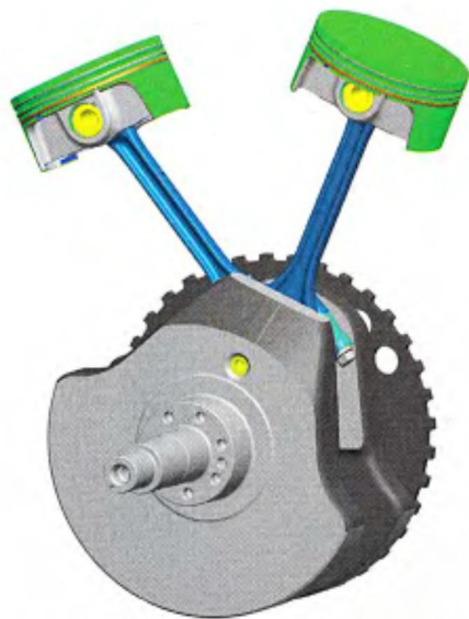
The one-piece forged crankshaft, connecting rods and pistons were CAD designed.
