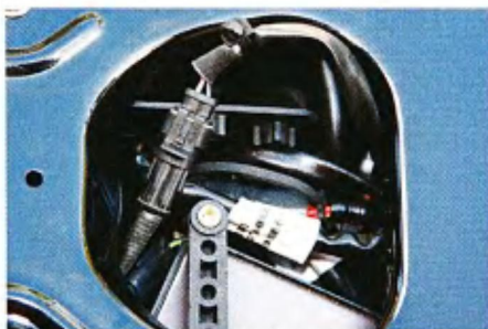
6 The connector for the rear oxygen sensor is in the wire harnesses under the seat. We found it by tugging on the wire down by the pipe and watching to see which connector moved in the cavity under the seat.
