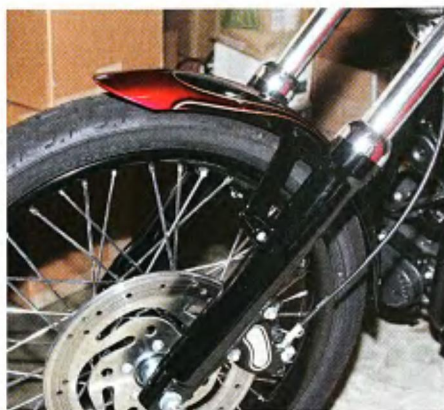
5 Installing the new front fender took about fifteen minutes.
