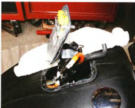
15 With the center cover raised up, you can remove the interior parts. This is where a service manual is needed; the parts must be removed in a certain order.
