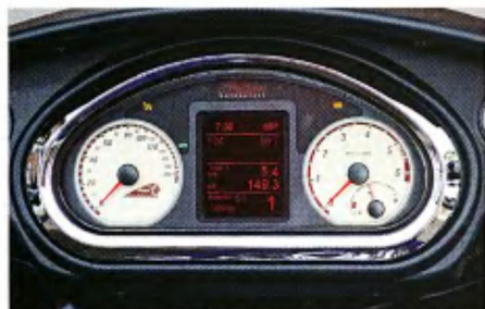
The business side of the Chieftain's fork-mounted fairing: it's all 21st century gages and audio, with a powered windshield.
