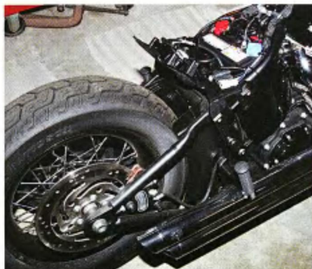
9 When the fender is removed, the fuel injection computer and all of its wiring remain on the bike.
