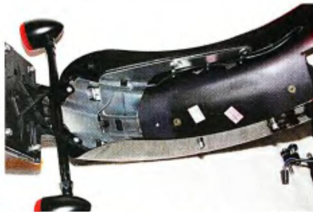
10 The taillight/license plate assembly is transferred to the new fender in one piece.
