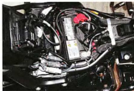
7 The rear fender required unplugging the taillight wire harnesses' three connectors.
