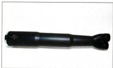
3 The muffler also has three steps, going from front to back. The Vance & Hines logo and chrome end cap is a nice touch.
