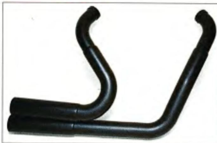
2 The head pipes have a three-step design. Their lower end fits into the front of the muffler.
