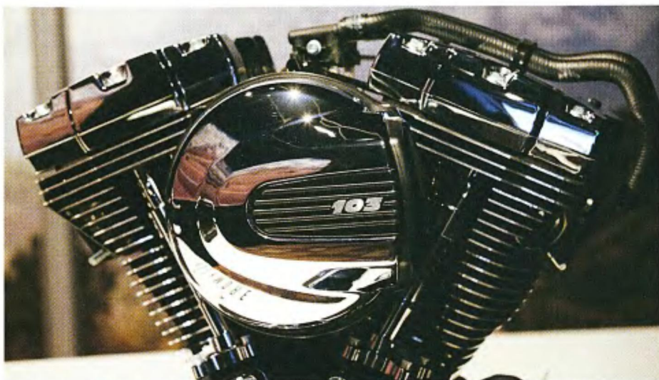
Harley-Davidson's new-for-2014 Twin-Cooled High Output Twin Cam 103-inch engine featuring liquid-cooled heads and a new air filter housing designed specifically for the Rushmore Project models.
