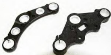
1 The stock Blackline top triple tree is on the left and the Todd's Cycle triple tree is on the right. With this top tree, you can run any type of handlebars.
