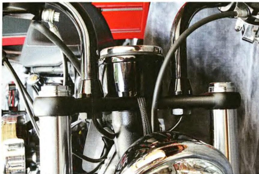
3 Each side of the factory bars is bolted directly to the top tree.
