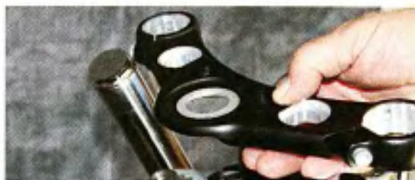
7 We put a bike lift under the frame and raised it just enough to take the weight off of the front wheel, and removed the top tree. Because the Blackline uses a steering head nut under the top tree, the fork did not loosen.
