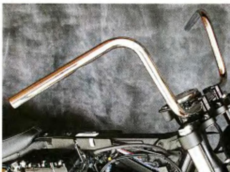
9 The Alloy Art risers and Flanders mini apes bolted right up to Todd's top tree. Once everything was put back in place, the bike looked and rode a lot better (below).
