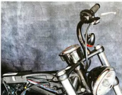
4 Taking the handlebars and controls off requires removing the gas tank.
