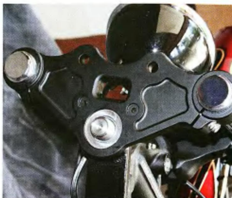
8 Todd's top tree was a direct replacement for the factory tree.
