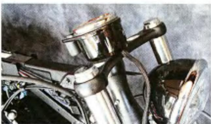
5 The speedometer and idiot light cluster are unplugged from the bike's main wire harness and unbolted from the top tree.
