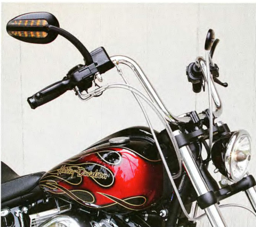
9 The Alloy Art risers and Flanders mini apes bolted right up to Todd's top tree. Once everything was put back in place, the bike looked and rode a lot better (below).
