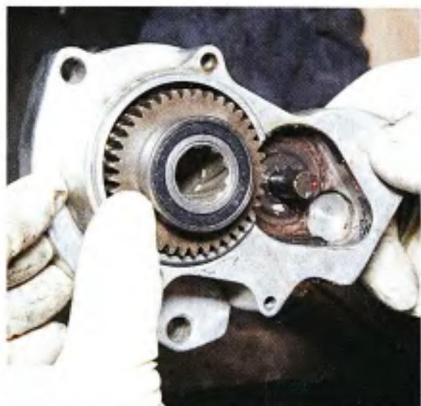
7 The new starter drive clutch assembly is coated with bearing grease and fitted into the nose housing. The starter's extension shaft is rotated counter-clockwise to fit it into of the drive clutch's center bore.
