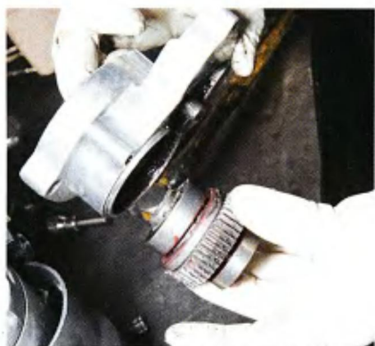
6 The starter drive clutch assembly is removed from the nose housing. In most cases it can be removed without using any type force.
