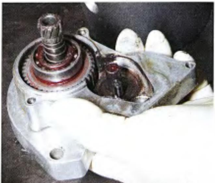
4 Next the nose housing is removed from the starter's main body.
