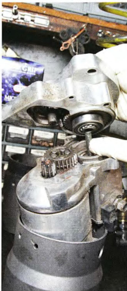
11 He did this while at the same time he was aligning the intermediate gear into its cavity. Believe me, doing this took a lot of experience!
