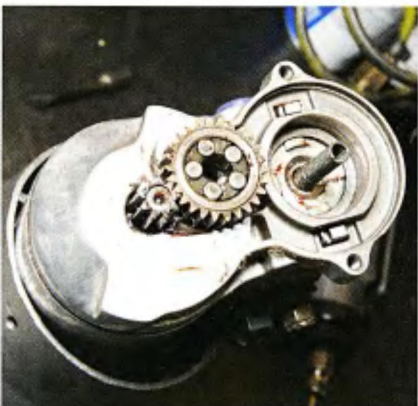
9 The intermediate gear is then fit up to the starter's pinion shaft, on the main body of the starter. This is something we would have done backwards, we would have set it into the cavity in the nose and then tried to assemble the nose onto the main body.
