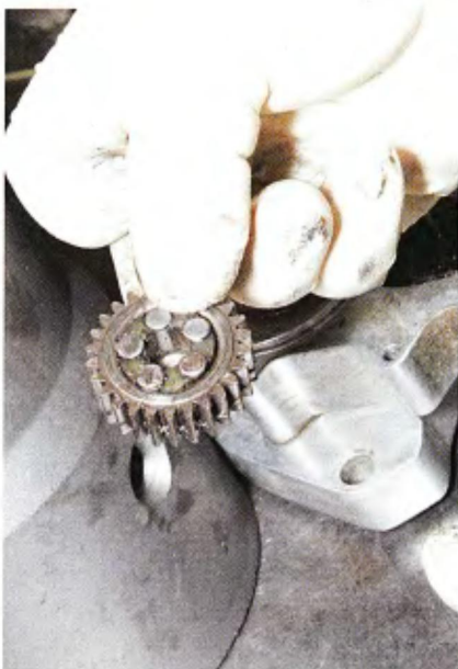
8 The starter's intermediate gear with its five rollers is lubricated.
