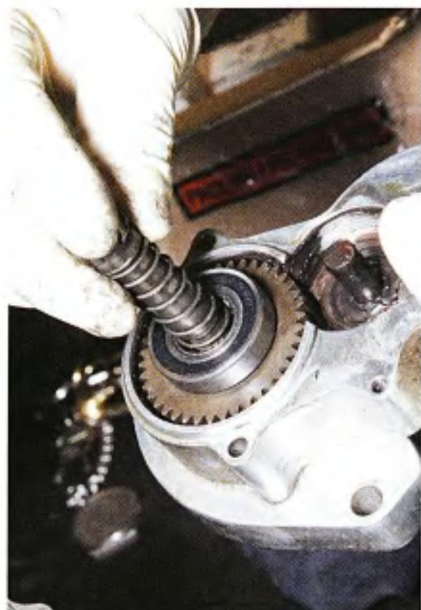
5 The starter extension shaft is rotated clockwise to pull it out of the drive clutch's center bore.
