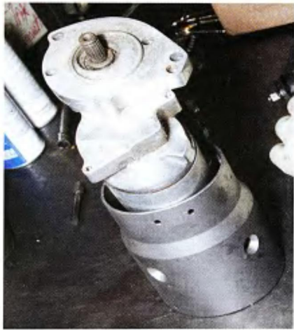
3 Oscar starts the repair by removing the screws that secure the starter's body to its nose housing.
