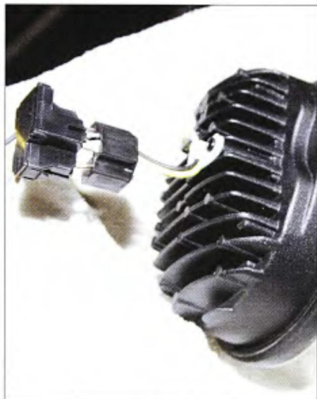
4 The LED headlight's wiring connector plugs directly into the factory wire harness.
