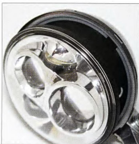
5 The LED headlight has a small tab on its right edge that fits into a recess in the headlight bucket's inner rim. The headlight is secured to the headlight bucket by a mounting ring that fits tightly over the edge of the light and the front of the bucket. It uses a single screw and nut for attachment.
