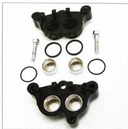
4 The calipers' bores, pistons and internal seals must be absolutely clean; the H-D service manual was a huge help in installing these parts.
