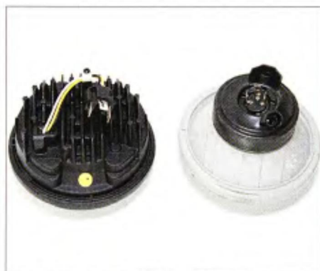
3 The rear of the headlights tells a similar story. To aid in cooling and strengthen the housing, the LED headlight has multiple polycarbonate fins. The regular headlight has a thin plastic shell that mounts a separate light bulb.
