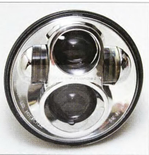
1 Harley's new 7-inch LED headlight has four groups of LEDs mounted in a cross pattern. Each LED group has its own lens and reflector assembly. The low beam uses the upper lens group and the high beam uses all four groups.
