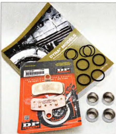
3 Along with the cleaned factory caliper pistons, we used new seals and DP brake pads.
