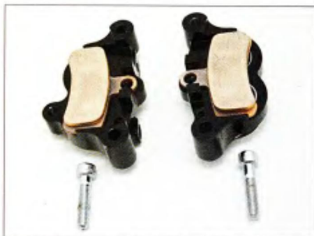
5 here is a transfer port O-ring seal that Ness fits into the rear caliper half, make sure it is still in the caliper body. The DP brake pads fit over the pistons.
