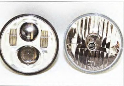
2 A side-by-side comparison of a factory Harley-Davidson halogen headlight (right) and the new LED unit (left) show the different designs used in its lenses and reflectors.
