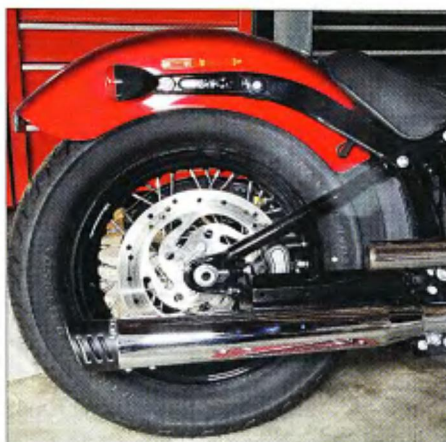
5 The Freedom mufflers bolted right up to the bike's factory mounting bracket. We also re-used the original muffer mounting bolts.
