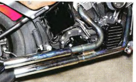
8 These Vance & Hines pipes have a secret. There is a chamber that connects the pipes. This gives them the low-rpm torque of a 2-into-1 system, yet the look of drag pipes.
