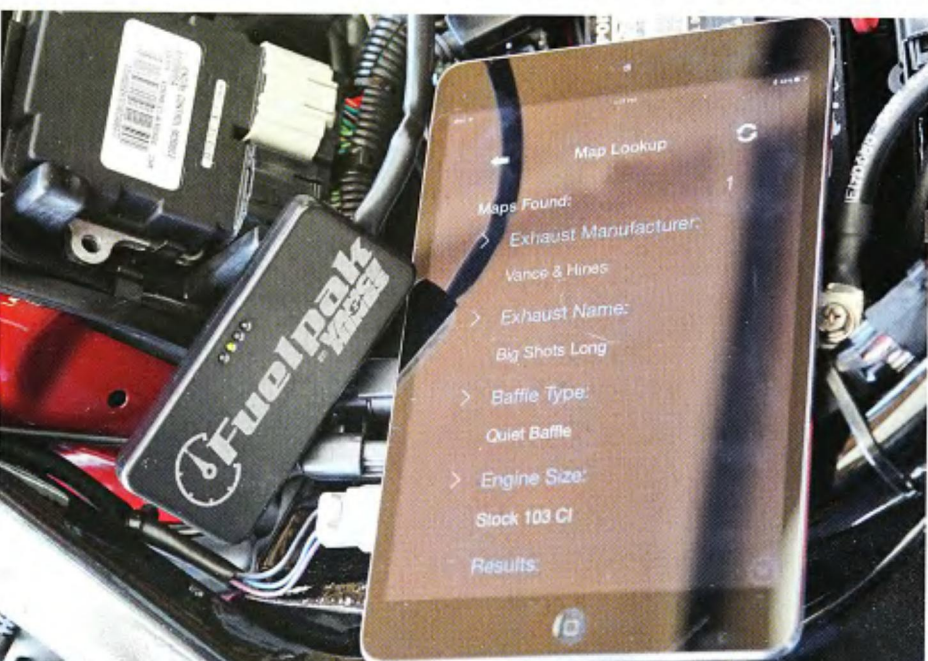
12 The FP3 communicates with the technician or rider through a Bluetooth device; we used an iPad. Once the iPad connected to the FP3, it displayed four apps. We used the "map lookup" to find the data to reflash the bike's ECM. We loaded the new fuel-management map with a touch on the iPad's screen and had ourselves a great running Softail.
