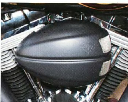
10 The air filter's black cover finished off the mechanical installations.
