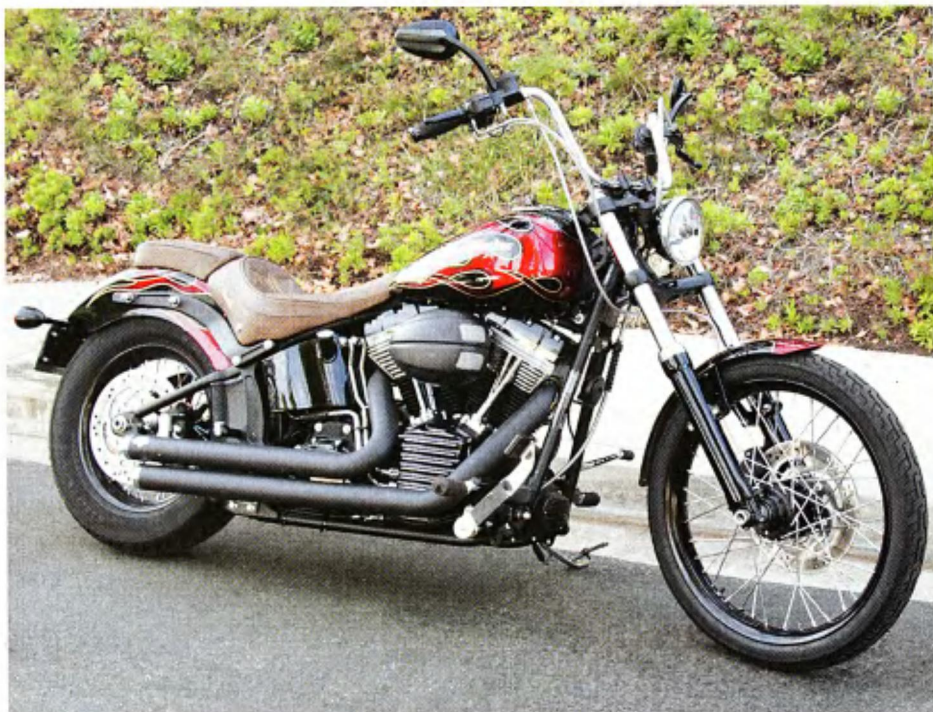
1 Our test bike is a 2012 Softail Blackline. We equipped it with the Vance & Hines Big Shot Staggered exhaust system, VO2 Drak high-flow air filter, and FP3 EFI tuning module.
