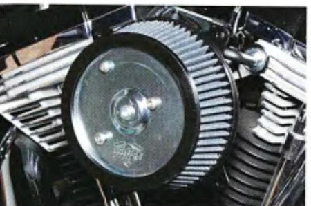
7 The filtering element is bolted in place. With the exception of installing the air filter cover, the air filter installation is complete.
