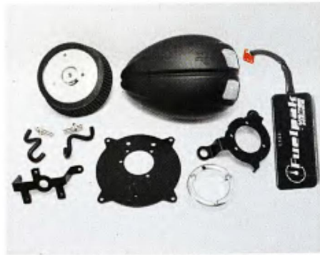
3 The Drak air filter kit is complete, and everything is a direct bolt on. The Fuelpak FP3 is just a black box with a wiring connector attached.
