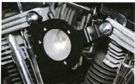
5 The Drak air filter's mounting plate is attached with the two engine breather bolts.
