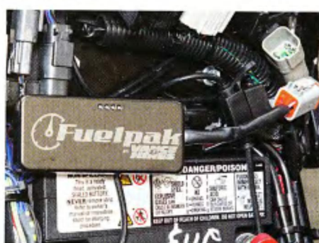
11 The FP3 module is a little larger than a business card; it plugs into the bike's VCI connector, which, on a Softail, is under the seat.
