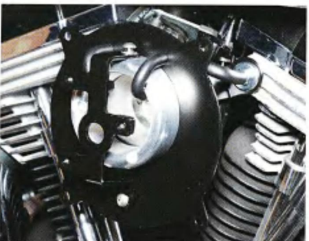
6 The air guide, breather hoses, and filtering element mount are installed.
