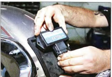
8 Installing the Dynatek module was just a matter of plugging in the bike's wire harness.
