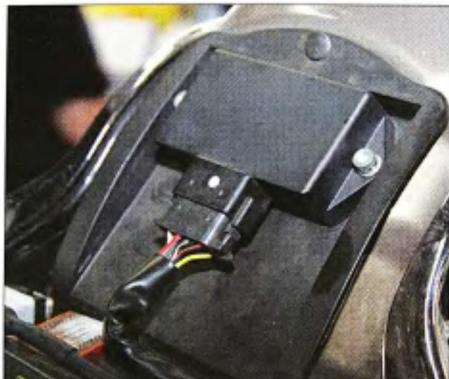
5 On the Fat Boy, the ignition module was located under the seat. Disconnecting the positive battery cable started the install.
