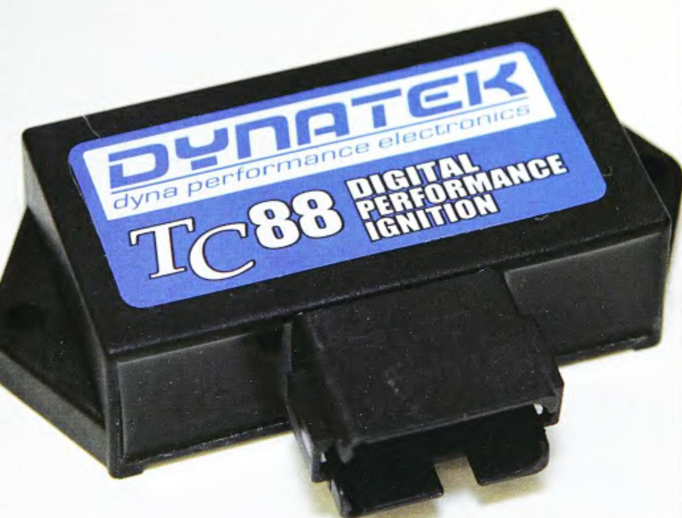
2 The module's rear edge has two small dials; one sets the advance curve, the other the rev limit. The included instructions have a clear graph of the setting used for most performance levels. The Fat Boy wound up with the advance curve set at 38A and a 6,250-rpm rev limit.
