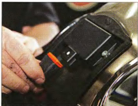
6 To install the module, the wire harness connector was unplugged from the stock ignition module. The two Allen screws were removed and the stock module was off of the bike.
