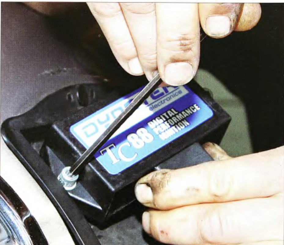
9 The new module mounted in the same spot as the factory unit, it even used the original mounting screws.
