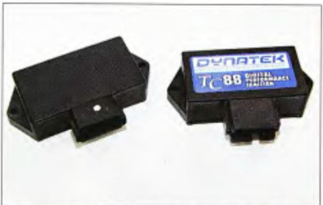
7 We set the stock ignition module and the Dynatek module were set side by side; they were the same physical size.
