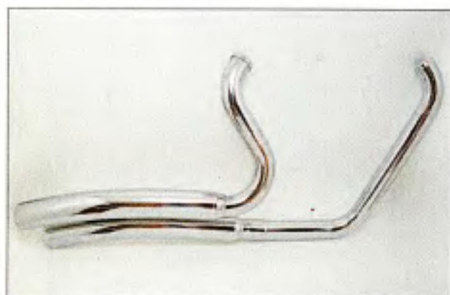
2 The system features a one-piece dual muffler with a hidden connector, which greatly improves the motor's mid-range performance.
