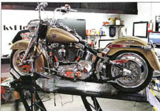
4 Our friend's 2004 Fat Boy had a performance exhaust and hopped-up carburetor, which the stock ignition system couldn't keep up with.
