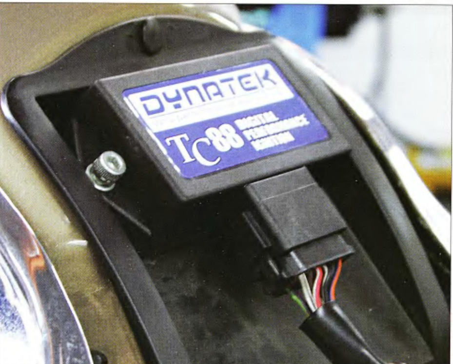
10 Because on the Fat Boy's ignition module mounts under the seat, it was really easy to get at to re-adjust it. Once the Dynatek module was dialed in, it didn't need further adjustments.
