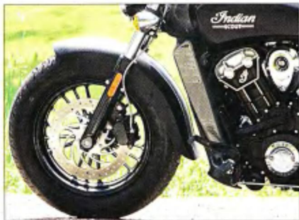
The 16-inch front wheel is fitted with a large diameter brake rotor and a multi-piston caliper.
