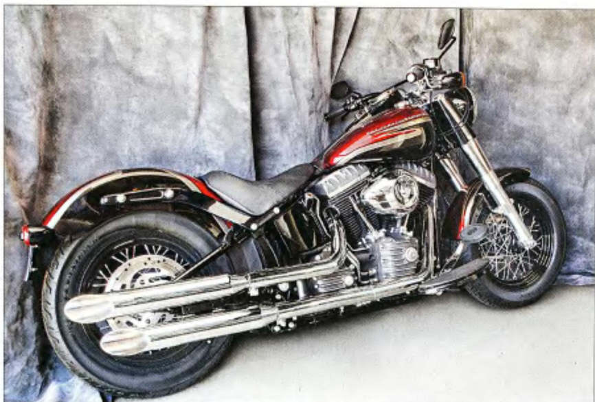
1 Here is our hopped-up Softail. The high-flow air filter and mufflers gave a boost in the torque, but the cams really kicked the power output upstairs.
