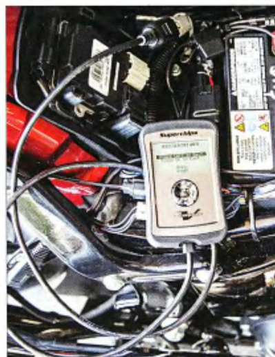
10 The Vigilante was plugged into the bike's Delphi ECM diagnostic connector; the handlebar run switch activated and we followed the prompts on the Vigilante's screen.
