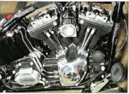
3 The starting point was a 2013 Softail Slim. It has Harley's 103-inch motor, which makes good power, but we wanted great power.
