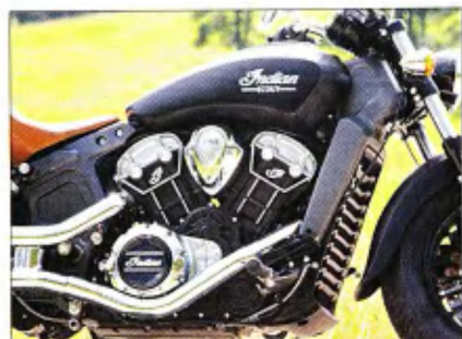
Although the motor is an overhead cam, liquid cooled unit, it is styled to appear like a pushrod type.
