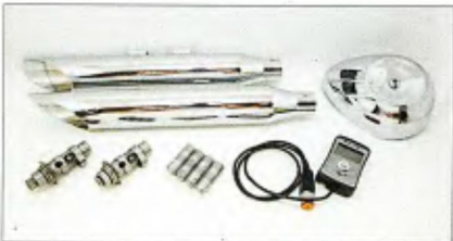
2 Our Power-Tune Kit consisted of: S&S's new MR103 cams, Premium hydraulic lifters, custom programmed Vigilante re-flash device, air stream air filter, and Slash-Cut slip-on mufflers.
