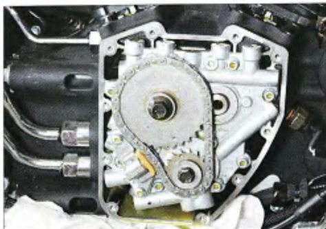
4 Installing a set of bolt-in cams requires going inside your motor, but not too deep. We removed the rocker covers, rocker arms, exhaust, air filter and cam covers.
