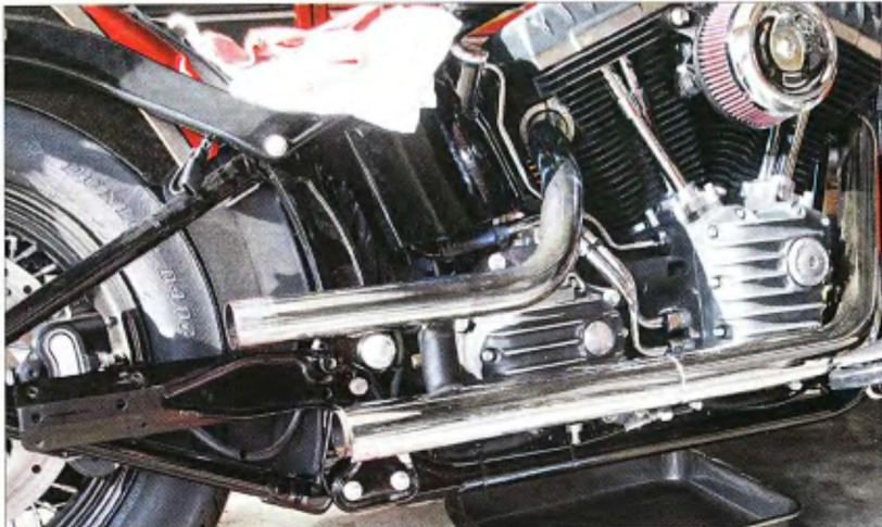
8 The stock exhaust head pipes were fitted to the cylinder heads.
