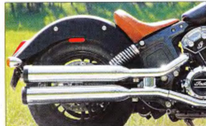
The shotgun exhaust system incorporates a cross-over port between its two head pipes.
