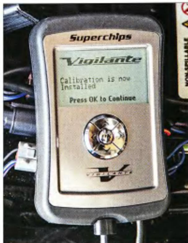
11 A few minutes later the Vigilante signaled us that the calibration re-flash was complete. We then rode the bike, which had a much sharper power curve; it felt like a real stump puller.
