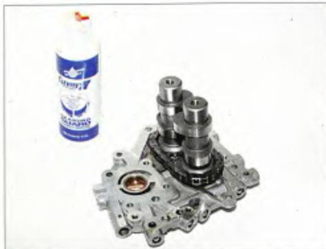
5 The new cams were installed on the cam plate with their timing marks lined up and the cam plate was fitted back on the motor. The new lifters and the stock pushrods were installed.
