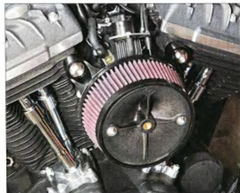
7 The air filter element and inner cover were fitted to the back plate.
