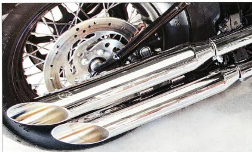
9 Installing the S&S Slip-On Mufflers completed the mechanical assembly of the bike.
