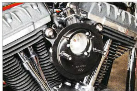
6 The top end of the motor was put back together and the S&S air filter's back plate was installed.
