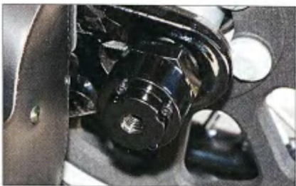
8 The Roto-Plate adaptor is secured with four Allen screws.
