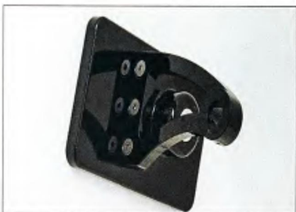
3 The kit's mounting bracket is secured to the Roto-Plate license mount with three stainless steel Allen screws, which have locking patches imbedded into their threads.
