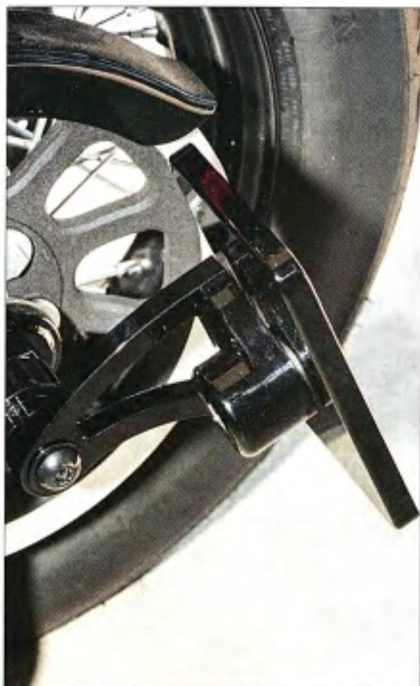
9 The Rotor-Plate mount is then attached with the included Allen bolt, which was torqued to 56 ft.-lbs.
