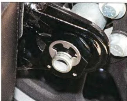
7 After the new axle nut was tightened, to 90 ft.-lbs., we installed the factory snap ring.
