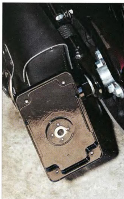
10 The center shaft of the Roto-Plate's hub is hollow for the license frame's wiring to run through. We spliced the license light's wires to the Slim's taillight wires.
