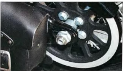
4 The Roto-Plate mount will be fitted onto the left side of the rear axle. This requires removing the locking snap ring and axle nut.
