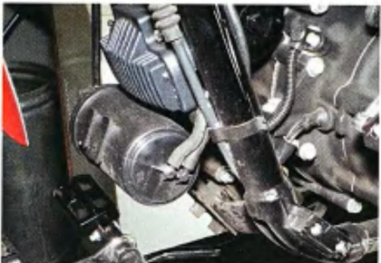
4 The gas tank's California-only purge canister was in the same place where the skid plate was going.
