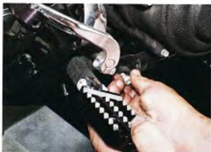
3 We started the install by removing the two Allen bolts that mount the left side foot controls, which we folded up and out of the way. We then did the same on the right side foot controls.
