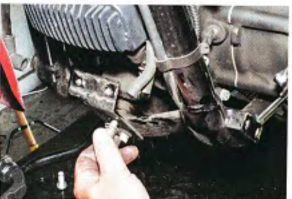
5 We removed the canister and relocated its intake hose up under the gas tank and ran it back to the rear fender. We then removed the canister's mounting bracket.
