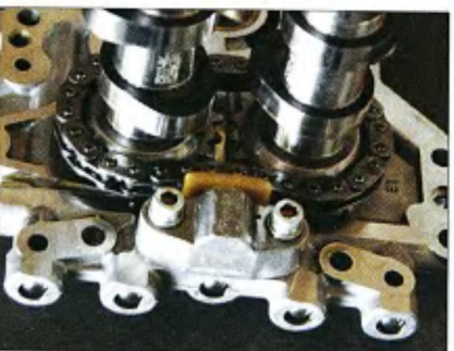
6 The cam plate was removed and flipped over; the inner drive chain tensioner is attached to the upper inside face of the cam plate.
