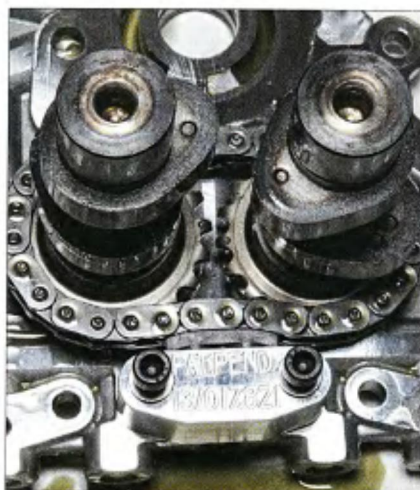
7 The new inner tensioner was installed on the cam plate. Both tensioners are direct bolt-on parts; no modifications to the cam plate needed.
