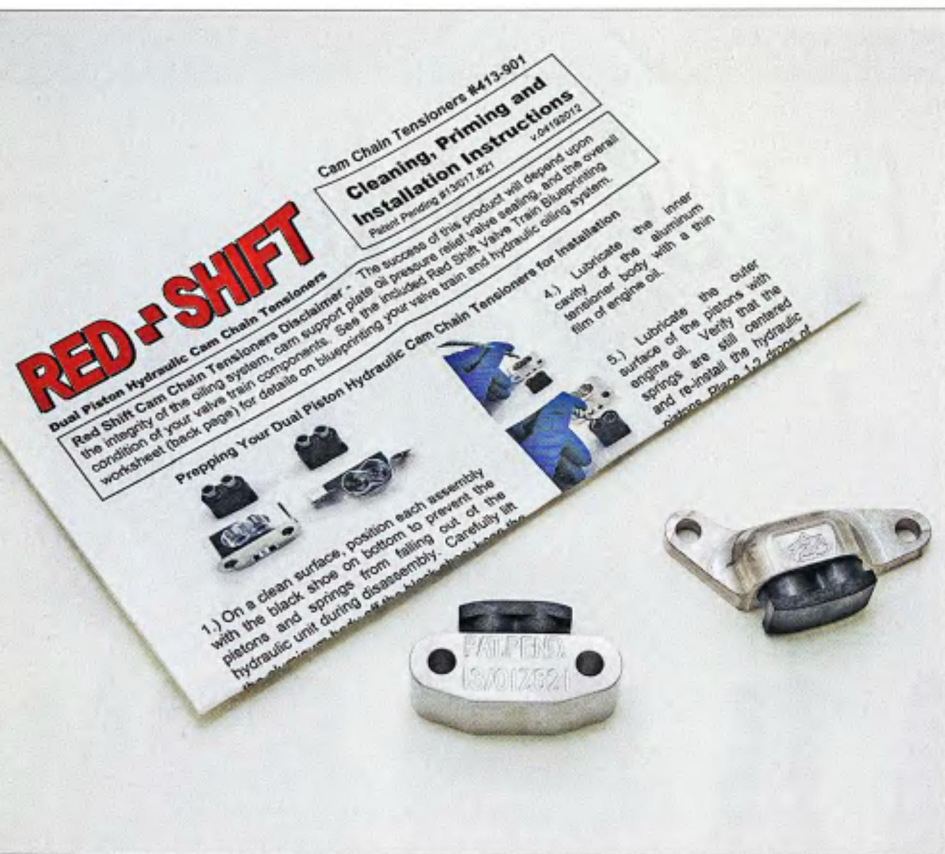
1 Zipper's Red Shift inner and outer cam chain tensioners are sold as a set. The housings are machined from billet aluminum and the shoes are injection-molded nylon.
