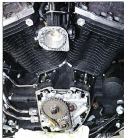
3 Installing the set of tensioners requires going inside your motor, but not too deep. We removed the exhaust system, air filter rocker covers, rocker arms, pushrods, valve lifters, and cam cover.
