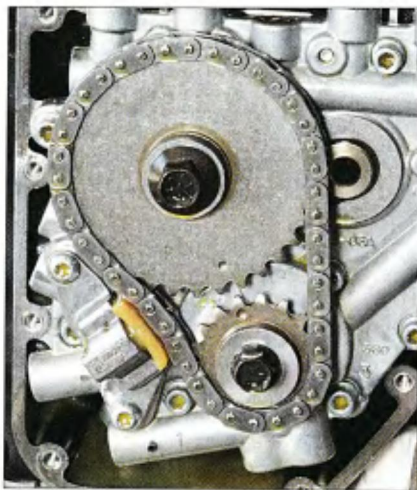
4 The stock outer drive chain tensioner is mounted on the front side of the cam plate. It is secured with two Allen bolts.
