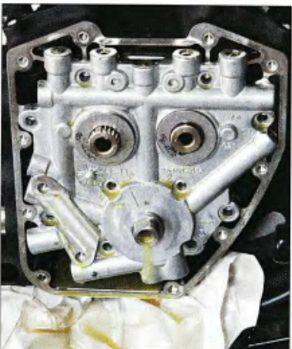
5 The cam drive parts were removed as well as the cam plate and oil pump mounting bolts.
