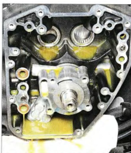
8 Before reassembling the motor, we carefully cleaned the cam chest and oil pump. We didn't remove the oil pump from the crankshaft.
