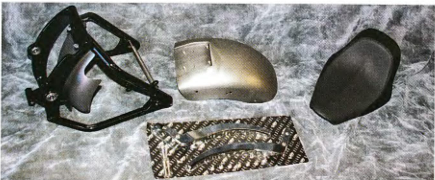
2 The basic 250 wide tire kit from Heartland USA. Looking over the new swingarm, we found the engineering and workmanship to be top-notch. The company has kits to convert 1986-up Softails to everything from 180 to 280 size rear tires.
