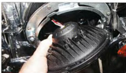
4 The LED headlight fits into the bike's stock headlight bucket.
