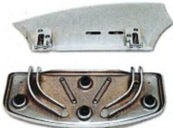
6 The benefit of the KewlMetal floorboards is not their only custom appearance. This is a comparison of the underside of the factory and the billet aluminum KewlMetal floorboards.
