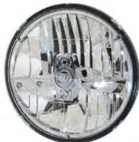
1 The LED headlight from Headwinds has five LEDs mounted in a cross pattern. Each LED has its own reflector setup. The low beam uses a single upper LED and the high beam uses the four mid-mounted LEDs.
