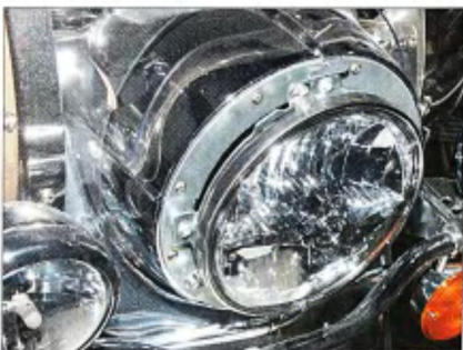
5 It reuses the factory mounting ring and bezel, which is secured with the three factory screws. And that's it, no wire cutting or soldering.
