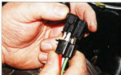
3 The connector on the wiring harness from the LED headlight plugs into the connector on the motorcycle's headlight wiring harness.
