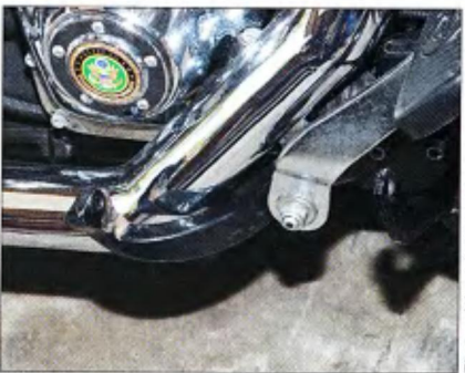
5 The KewlMetal floorboards fit onto the factory mounts without modifications.
