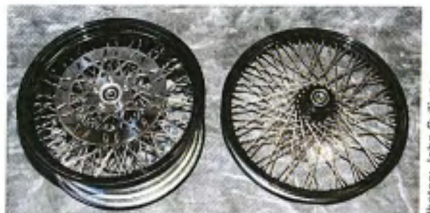
5 The Ride Wright wheels feature black hubs and rims with 80 chrome spokes.
