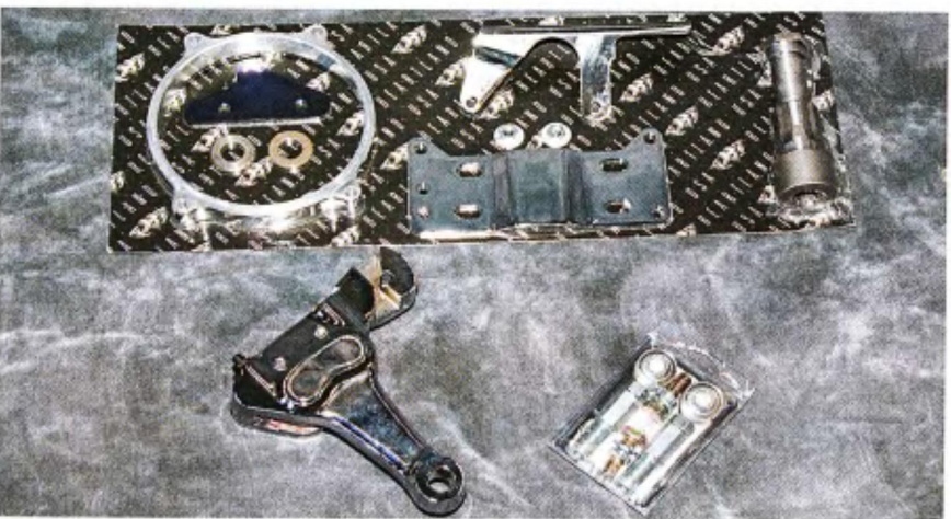
3 The kit includes an offset primary kit and rear brake caliper.
