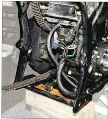
1 The starting point for our First Prize is a 1990 Softail Custom. Ed at My Garage has pulled off the rear wheel, fender, and swingarm.
