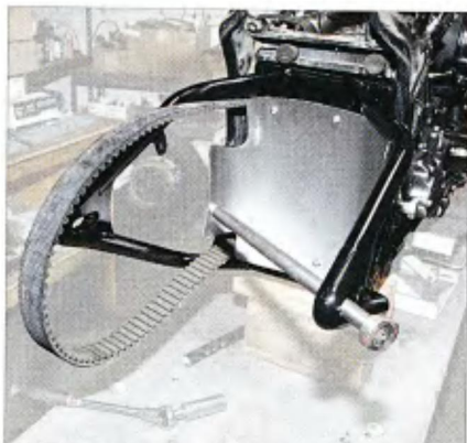
4 The Heartland swingarm went in place without any force or prying. We will need to cut off the rear fender struts.
