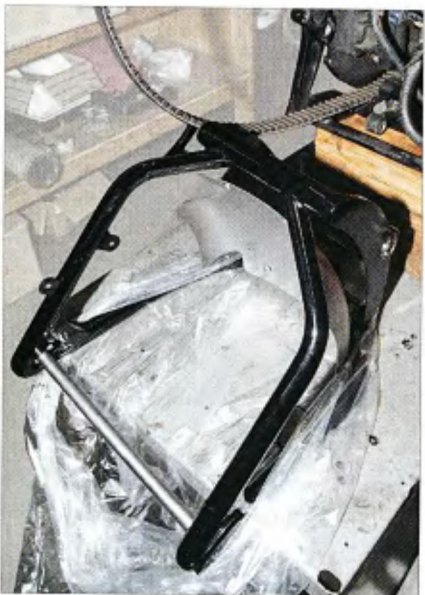
2 The Heartland swingarm is a work of art and its finish is flawless. It will fit into the stock Softail frame without any cutting or welding.
