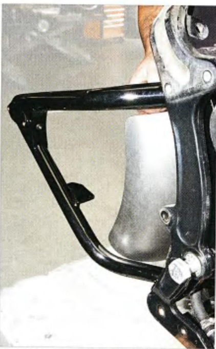
3 The swingarm was mounted with the factory bolts and swingarm mounting tube.
