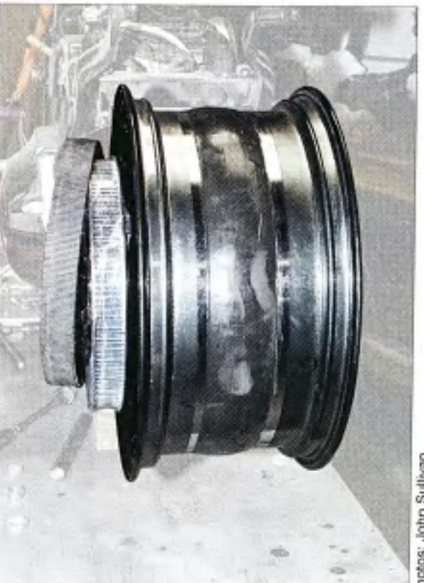
6 To allow the use of a tubeless tire, the Ride Wright wheel has a sealed spoke mounting center section.
