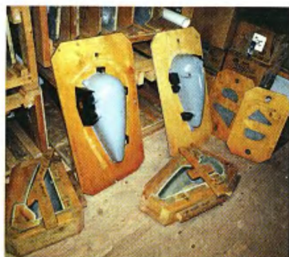
Six of 13 casting patterns needed for the Crocker gas tank.
