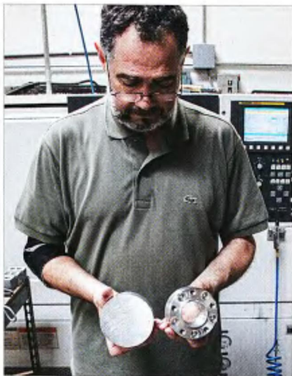
2 Sam's shop, Ridewright Wheels, does it all. In Sam's right hand is a billet aluminum blank and the left is holding a finished hub. He is standing in front of one of his six CNC machines that make not only the hubs but also spoke nipples, spacers, brake rotors and complete billet wheels.
