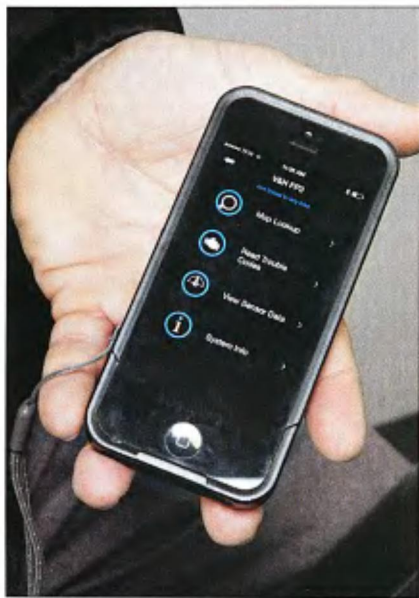
The FP3 connects to an Apple or Android device via Bluetooth; you don't need a PC computer to re-flash your bagger's ECM.
