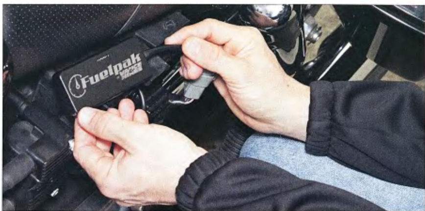
Vance & Hines new Fuelpak FP3 is a small electronic ECM re-flash device that plugs into the bike's VC1 data port. The FP3 operates with the stock 12mm O2 sensors.
