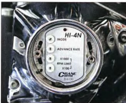
For older bikes that have separate ignition systems, Crane offers a couple of ignition controllers that let a rider tailor their ignition system through multiple adjustments.
