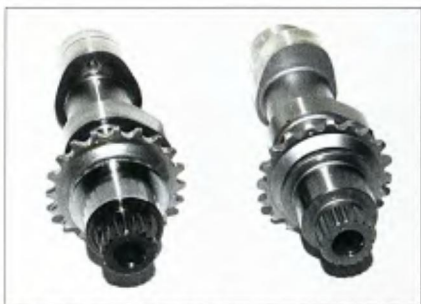
The stock camshaft (left) is very mild; the performance camshaft (right) will add a considerable amount of torque to your bike's motor. Selecting performance camshafts should be done very carefully because they control the rpm band where its torque output begins and drops off.
