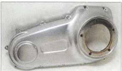
8 Harley's brushed-chrome parts not only look sharper than polished aluminum, they are also more durable.
