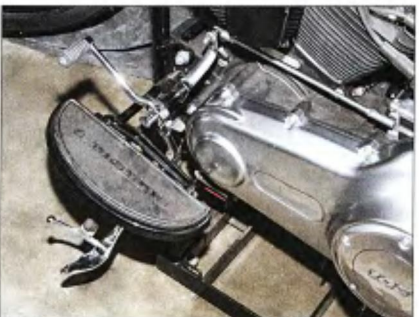
5 The stock floorboards are all right for baggers, but custom bikes need forward controls.
