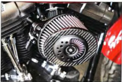
4 The RSD Slant air filter not only supplied more air to the motor, it also kept out of the way of our right knee.
