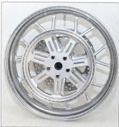
13 The rear wheel's pattern matches its pulley perfectly.
