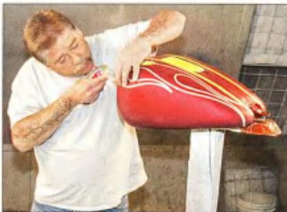
10 Vince at Conejo Auto Body gave the tank's stock red paint a light sanding, then started masking the tank in a flame design.
