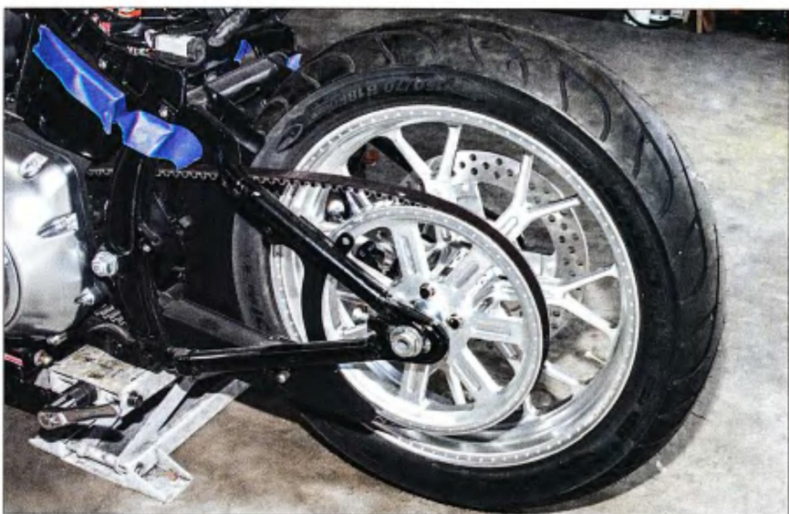
15 The 150- x 18-inch tire and 4 1/4-inch wheel fit right into the Slim's swingarm.
