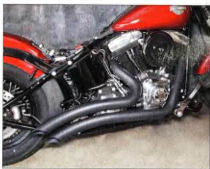
3 One of the first things we did to the bike was install a set of Cobra Speedster Short pipes, which work great.
