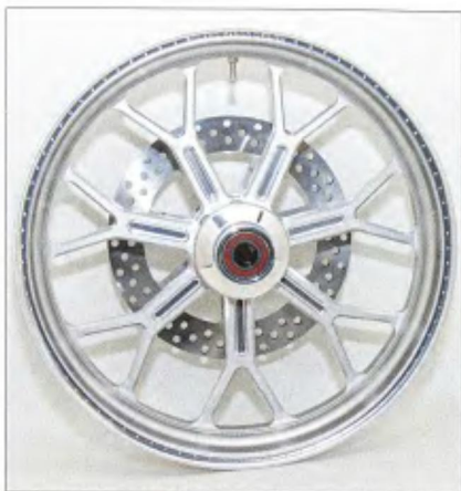
12 The RSD Del Mar wheels are machined from solid billet blanks. This front wheel weighs way less than the 16-inch spoke wheel.
