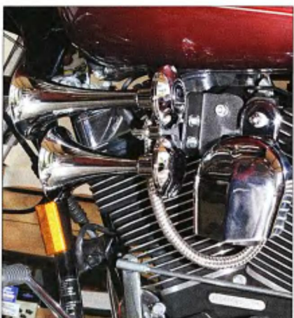
6 The completed horn assembly mounted on the bike; it is a well thought out kit.
