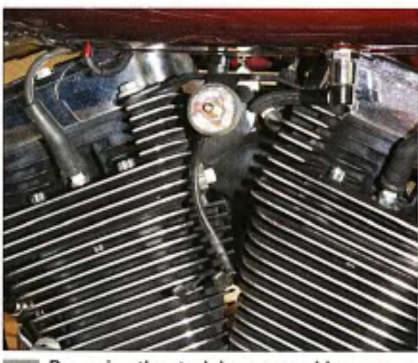
3 Removing the stock horn assembly was a 2-minute job, a 1/2-inch nut, and two wire connectors.
