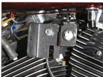
5 The horn-mounting bracket fits onto the stock horn isolator mount. We mounted the horn relay under the seat; its 12-gauge power wires were attached directly to the battery's terminals.
