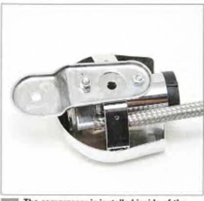
4 The compressor is installed inside of the factory horn cover. The air hose comes with its metal sheathing installed; we slipped the end of the hose onto the compressor's output fitting and tightened the hose clamp.
