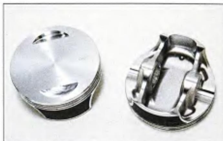
2 The forged pistons have flat tops and moly-plated skirts. When used with the Revolution Performance Stage 2 cylinder heads, they produce a compression ratio of 10.5:1.
