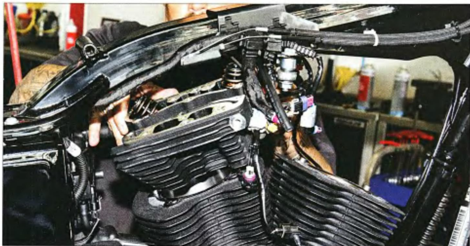
10 The Stage 2 cylinder heads were installed and their head bolts torqued down.
