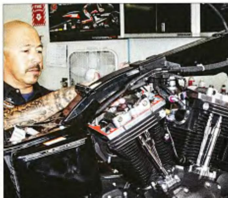
14 The rocker arms and their supports were installed and torqued down.
