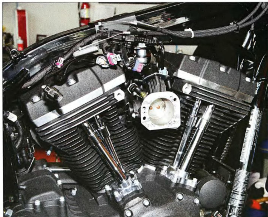
17 The completed motor didn't give a clue to its hi-performance internal components. We finished the motor with the stock exhaust head pipes fitted with a set of Screamin' Eagle slip-on mufflers and a Screamin' Eagle air filter.
