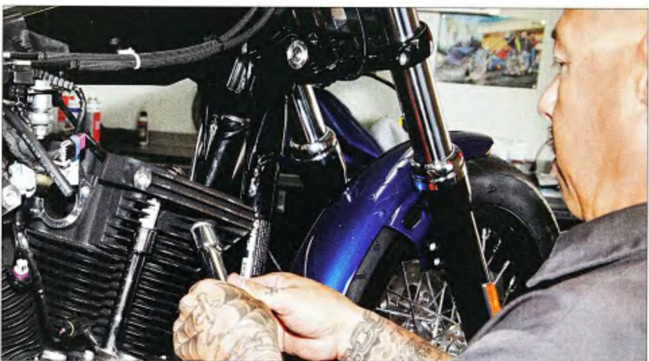
11 The pushrod tubes were fitted between the crankcase and cylinder heads.
