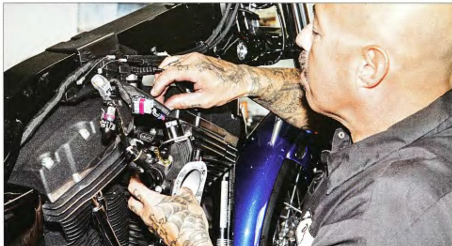
16 The throttle body and all of its control wiring were installed.
