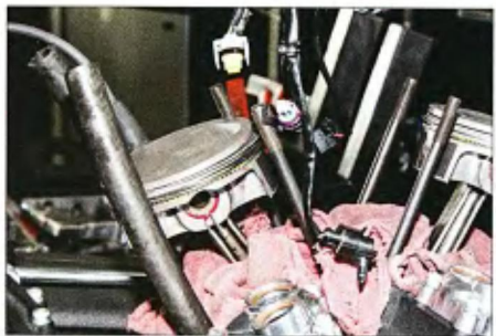
8 The piston rings were sized to the new barrels and fitted on the pistons. The pistons were then fitted over the top of each connecting rod and their wrist pins and locks installed.
