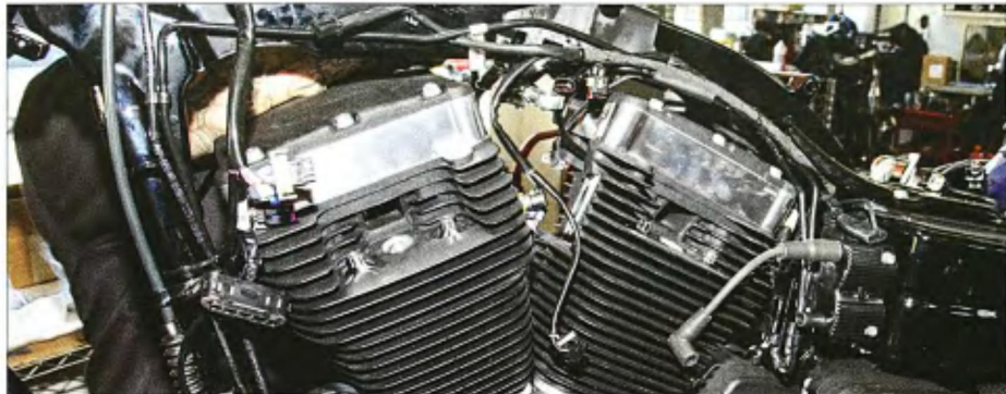
15 The rocker covers and the cylinder heads' electronic sensors were installed.
