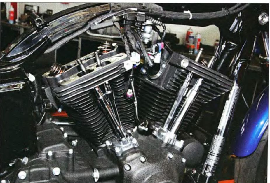
12 The stock pushrods were dropped into the cylinder heads and pushrod tubes. They were used because the No. 57H cams have a smaller heel diameter than the stock cams, which was offset by the cylinder heads being milled .020 inch.
