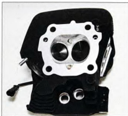
3 The Stage 2 heads are fitted with a 1.900-inch intake and 1.615-inch exhaust valves, a set of .650 lift beehive springs, and are milled .020 inch.
