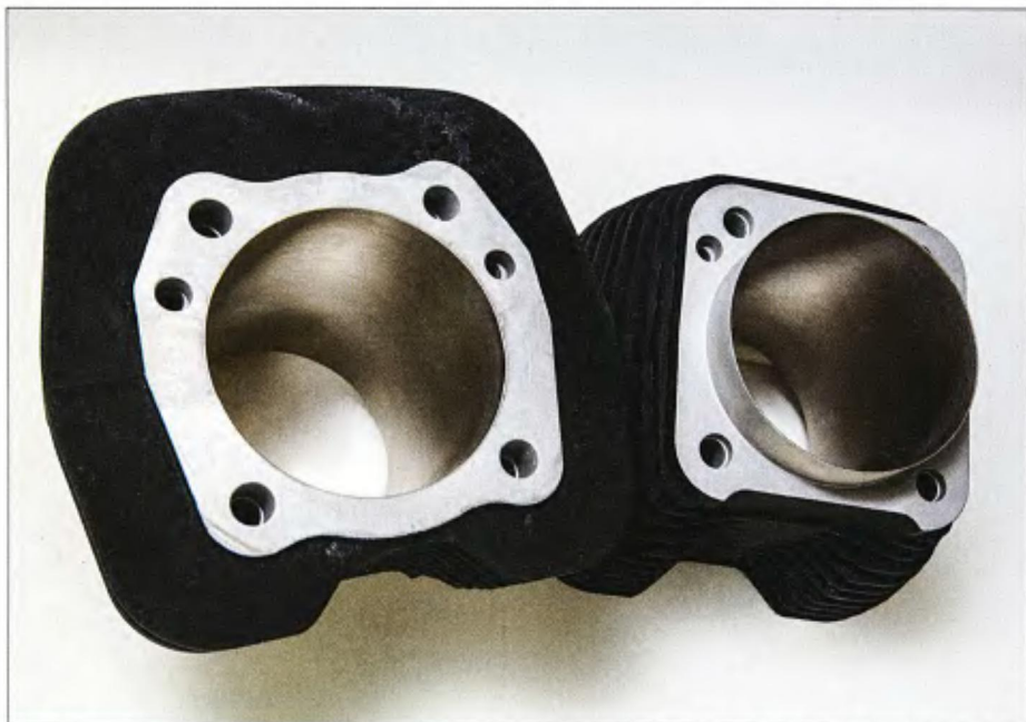
1 Revolution Performance's cylinder barrels are cast from aerospace-grade aluminum and then given a special nickel-silicon carbide-plated bore.
