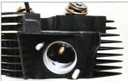
5 The exhaust ports were also CNC machined and like the intake ports, they were fitted with new bronze valve guides.
