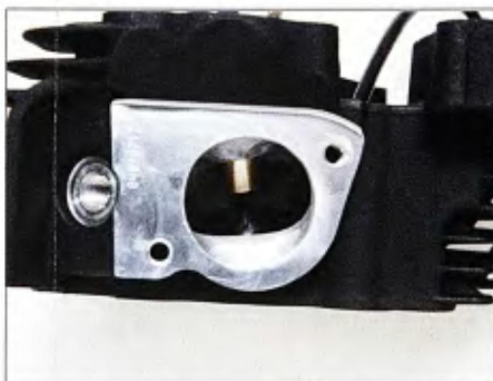
4 The intake ports were CNC machined to open up the area behind the valve seat.
