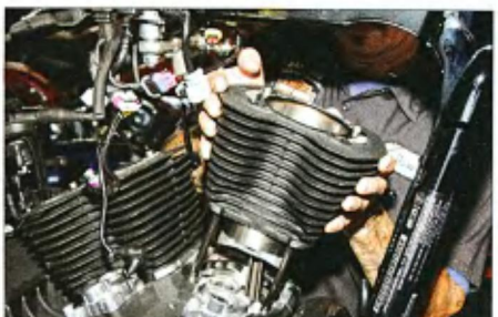
9 The pistons were fitted with a piston ring compressor, then the cylinders pushed down over them.
