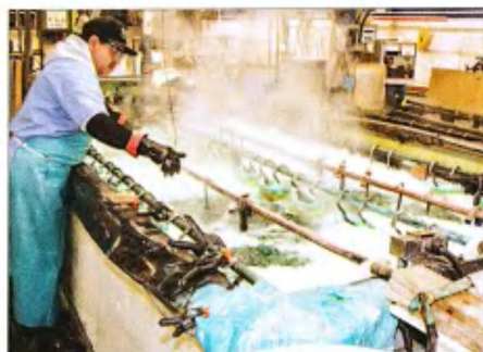
6 The super cleaned heat shields were then nickel-plated. The nickel acts as a bonding agent for the chrome plating.
