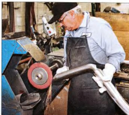
3 Next, the heat shields' outer surfaces were smoothed with a fine grit abrasive wheel.
