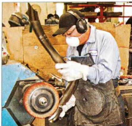
7 The nickel was then given the brushed surface finish.
