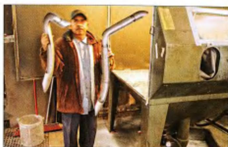
2 The first step in the re-finishing process was to bead-blast the original black finish off of the Cobra heat shields.
