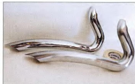
11 Here's a side-by-side comparison of our brushed chrome heat shields and regular bright chrome plated ones.
