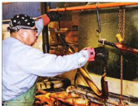
8 Once the prep work was finished, the heat shields were finally chrome plated.
