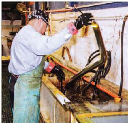
9 The excess chroming solution was then washed off of the heat shields.
