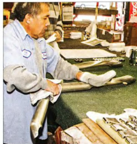
10 The final operation was a hand cleaning and a thorough quality check.
