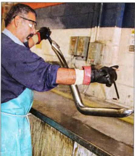
4 Then the cleaning started, they washed them in three different tanks.
