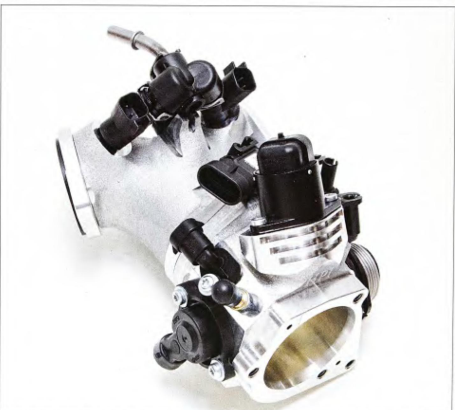
17 With the installation of the injectors into the throttle body, its bench work was completed. Now we just reversed the process that we had used to remove the factory throttle body to install the Horsepower unit. Then it's just a matter of installing the gas tank and firing up the motor.
