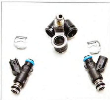
16 The new injectors were fitted into the fuel manifold and their locks slipped into place.
