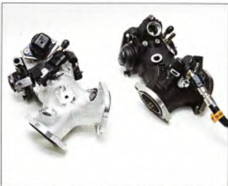
14 Removing the injectors and their manifold was a bit more work; the bolt that secures the manifold to the back of the throttle body had a ton of thread locker on it.
