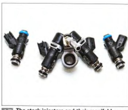
15 The stock injectors and their manifold came out as a unit. Except for the blue O-rings, the new injectors look just like the factory ones.
