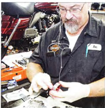
7 Ron started the install process by lubing the camshaft's lobes and bearing journals, and then he lubed all of the oil pump's internal parts and put it together.
