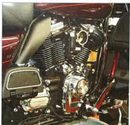
3 The install started with the removing of the air filter, right-side floorboard, and exhaust system. Ron then pulled the pushrod tube retainers, then cut the pushrods in half with bolt cutters and removed them. 110-inch motor needs. The throttle blade on Horsepower's 55mm throttle body (left) has 50% more area, which gives the motor a real kick in the mufflers.
