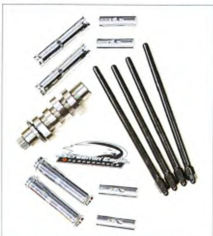
2 These are the parts that will improve power: a Screamin' Eagle camshaft and adjustable pushrods. Along with these parts, the motor's EFI computer will need to be updated with a new map.
