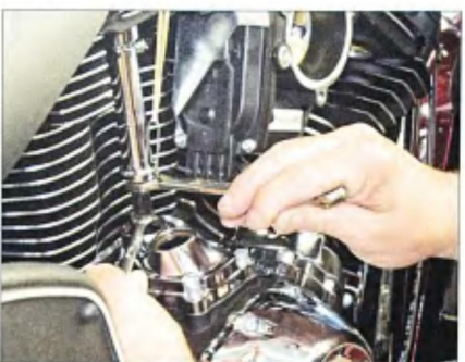
12 The final operation on the motor build was to install the pushrods and adjust the new pushrods. Then it was just a matter of fitting the air filter, exhaust system, and floorboard.
