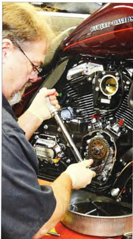
11 Ron used new camshaft and crankshaft sprocket bolts and torqued them down. When tightening these bolts, the Milwaukee-Eight motor uses the same sprocket-locking tool as is used on Twin Cam motors.
