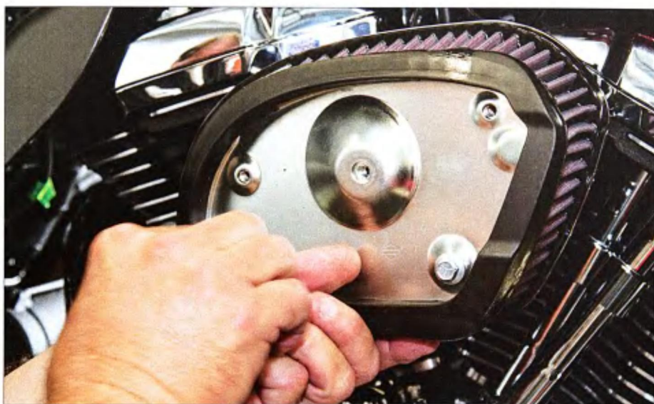
12 The new SE high-flow filtering element was fitted over the back plate.
