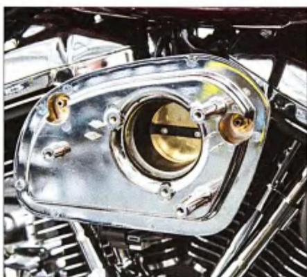
8 The back plate was also attached to the motor's cylinder heads with the two special breather bolts.
