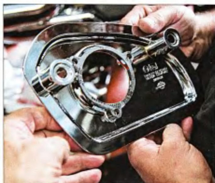
6 The high-flow air filter kit's cast aluminum back plate and throttle body gasket were assembled together. The new self-sticking gasket was applied to the backside of the SE back plate.
