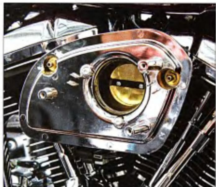
10 The SE back plate perfectly fit the throttle body and its outlet has a smooth radius into the throttle body's bore for better airflow.
