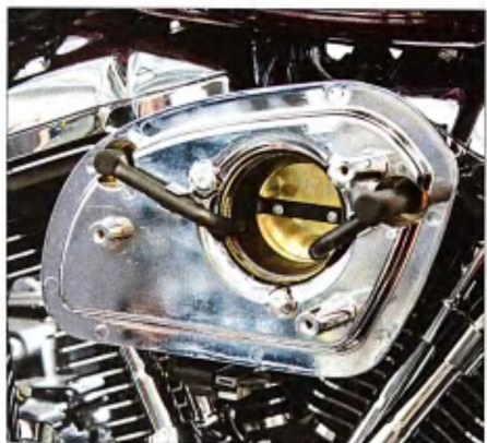
11 The breather hoses were fitted over the breather bolts and into the inlet of the throttle body.
