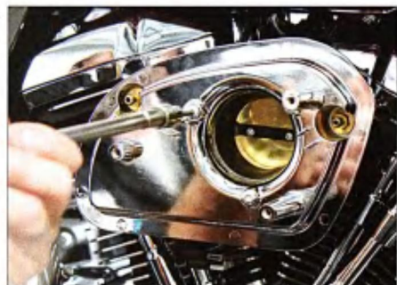
9 Once the back plate was aligned, the throttle body screws and breather bolts were torqued down.
