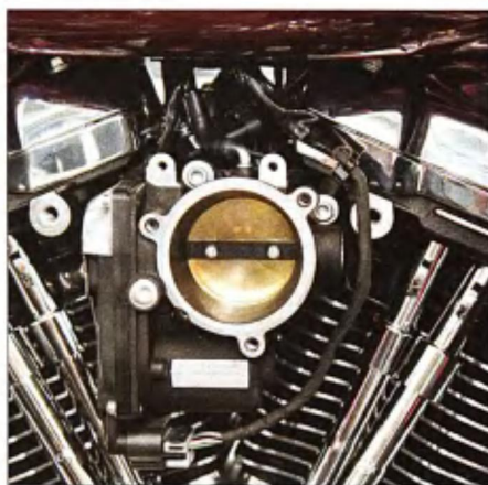
5 The throttle body-mounting bracket was also removed; its mounting bolts weren't reused.
