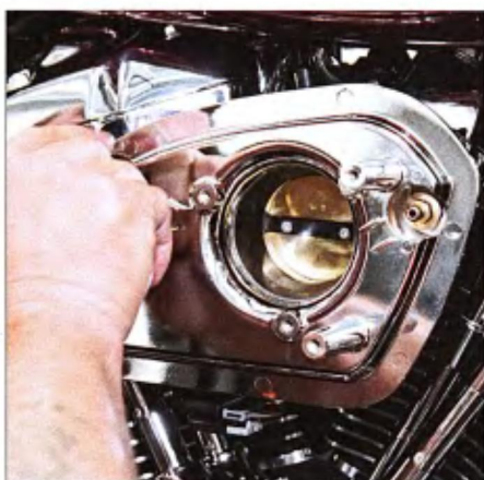
7 The back plate was loosely attached to the throttle body with three included Allen bolts.
