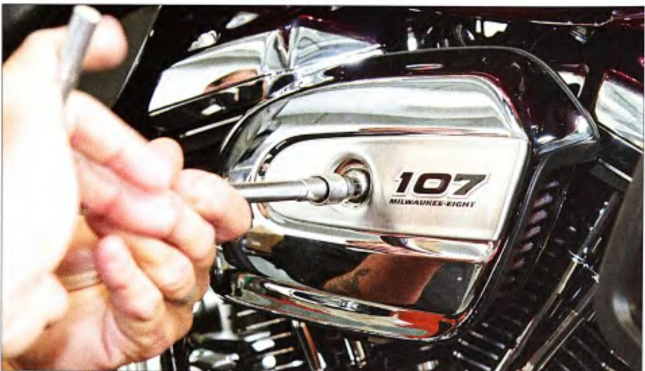
14 The final operation was to install the stock air filter cover.
