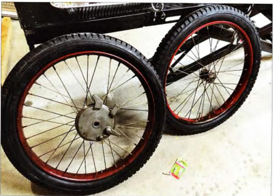
Clincher wheels were originally used on bicycles, early motorcycles and carts with a top speed of 30 miles per hour.
