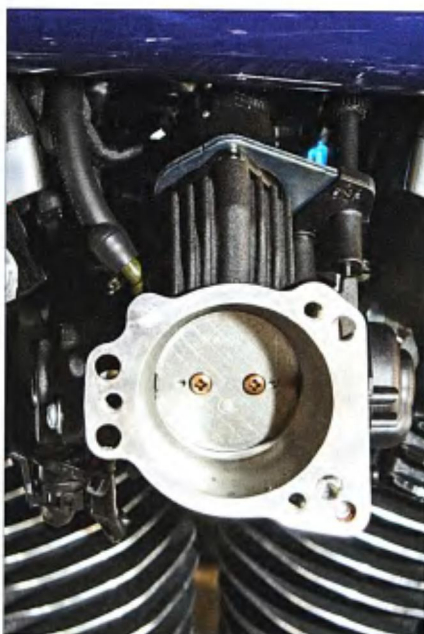
4 For our starting point, we have removed the stock air filter and its housing.
