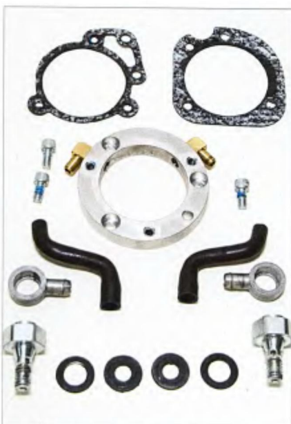
3 The other sub-assembly is the cylinder breather system; it feeds the motor's oiling system residue into the throttle body throat.
